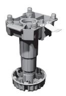
Base and tall units are supplied with height adjustable feet. The adjustment range from + 20 to - 10 mm guarantees millimetre accuracy. The plinth panel is protected against moisture by a sealing or
