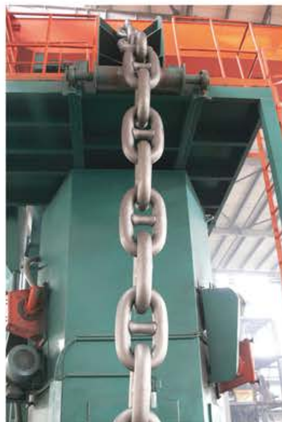
抛丸机 shot blasting machine
