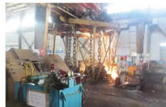
预热连续闪光对焊机组 Preheat continuous flash butt welding machine
