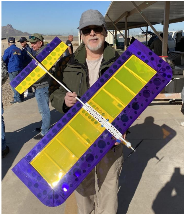
Right, Steve scratch-built this two-motor, contra-rotating propeller system. Amazingly complex. Steve did it with a CNC machine.
