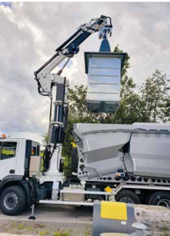
SPEED-WASTE-LIFTER: Long ranges, high stroke.
