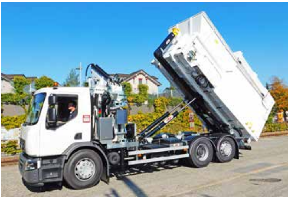
Operation of the Safety two-hand control for the tailgate.
