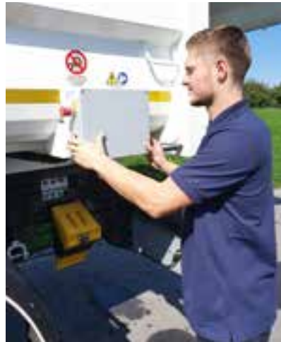
Operation of the Safety two-hand control for the tailgate.
