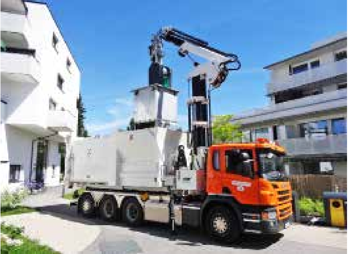
4-axle vehicle with hooklift and SPEED-WASTE-LIFTER 105-7 with compacting press VCP 18
