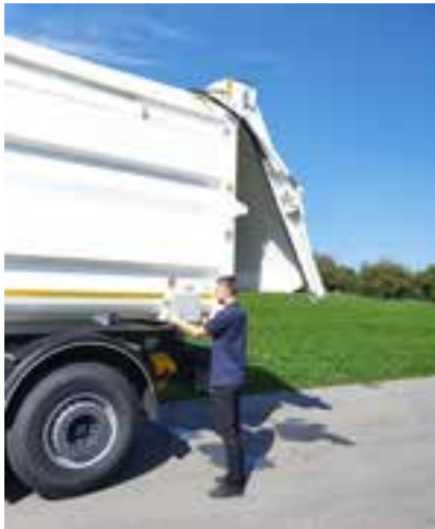
Operation of the Safety two-hand control for the tailgate.
