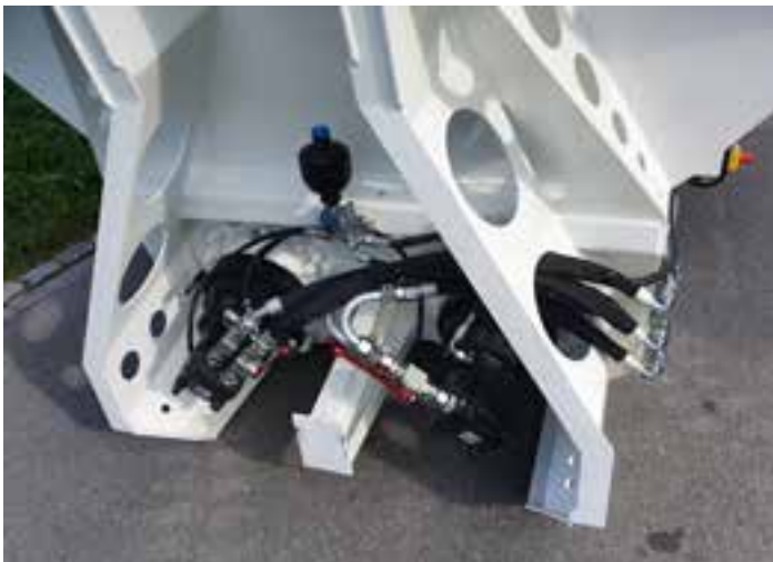
Hydraulic oil transmission motor
