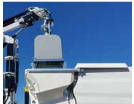
Roof opening with hydraulic closure
