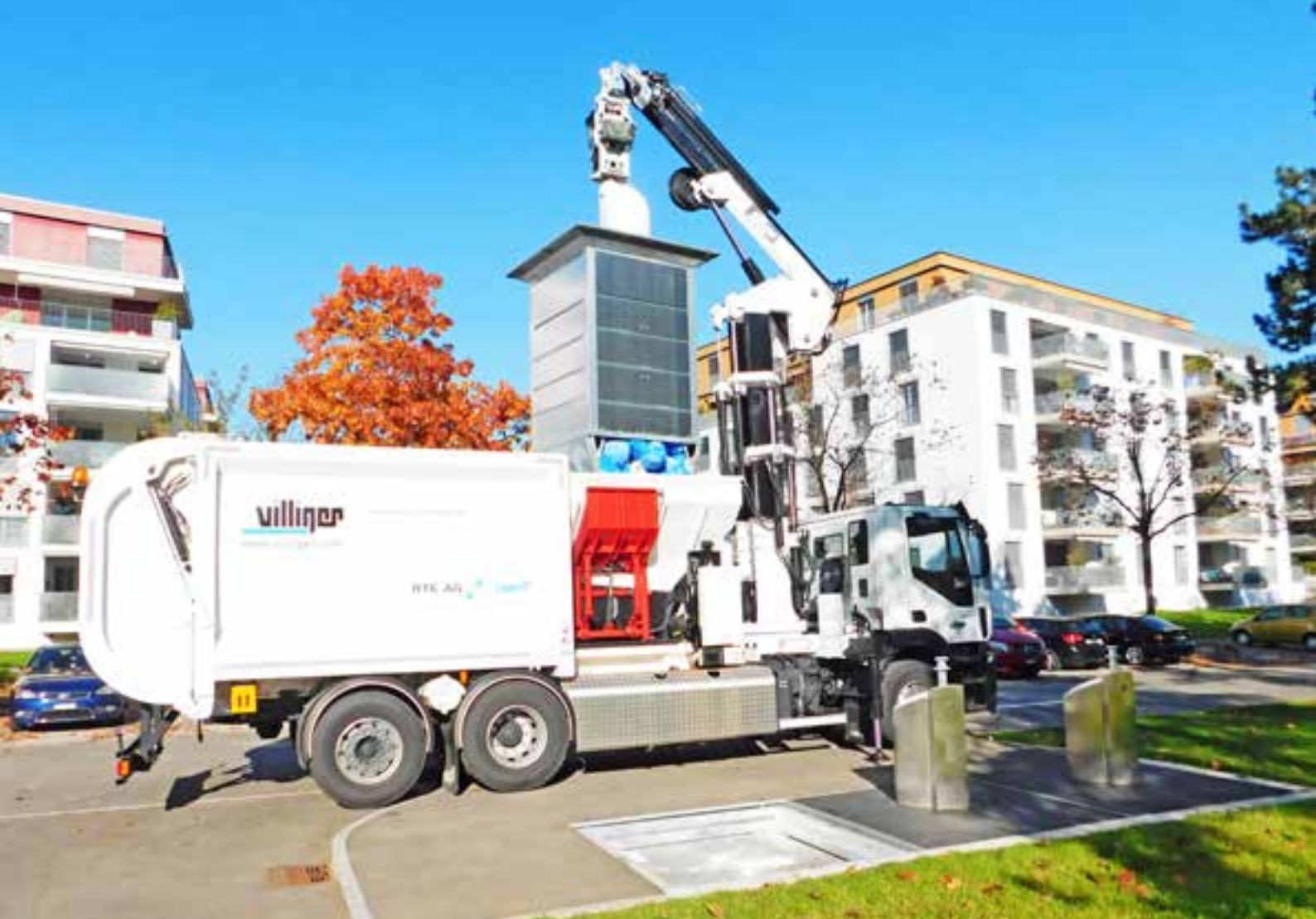
3-axle waste disposal vehicle with SWL 105-7, a collecting compactor with 18 m 3 capacity and a bag trough.
