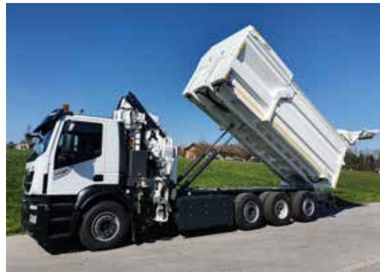
4-axle vehicle with fixed compactor and SWL 105-9.
