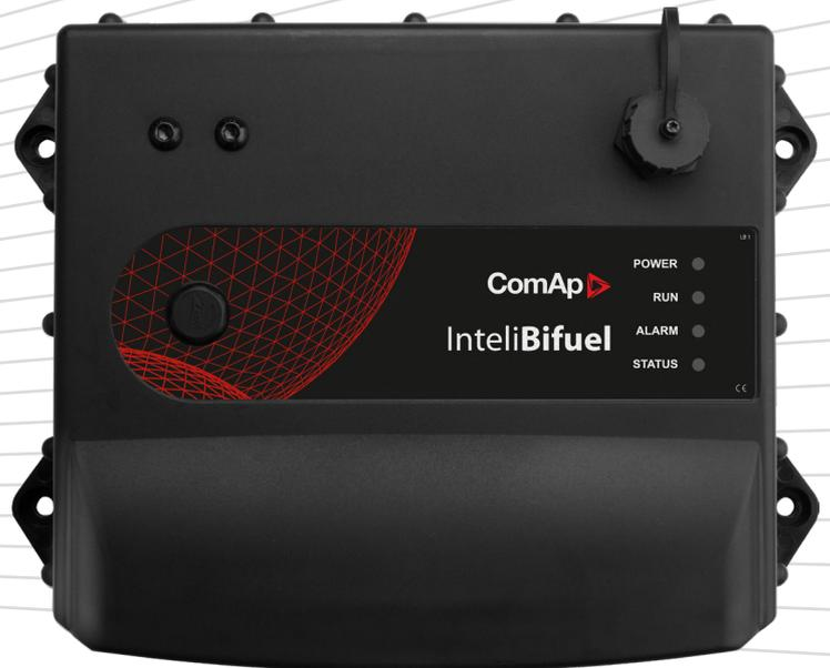
ComAp's simple bi-fuel conversion modifies your original diesel power generation engine so that it uses natural gas as the main fuel - substantially reducing operating costs. It works by introducing gas into the engine and then electronically controlling gas flow dependent on engine speed and output.
