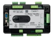
> A Mains Supervision Controller Base Unit with Extended Communications for Use with Detachable Colour Display
