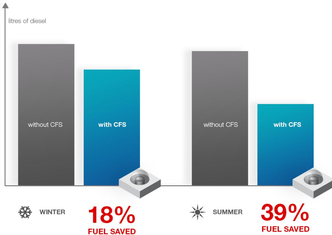
\* Results of a case study from production facility with industrial load profile and 375 kVA diesel generator connected in parallel with a 1MWp PV plant. Location: California. Solar output data source: NREL
