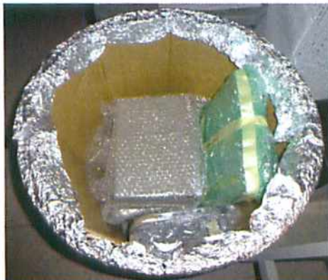
Put wrapped & insulated equipment in galvanized container
