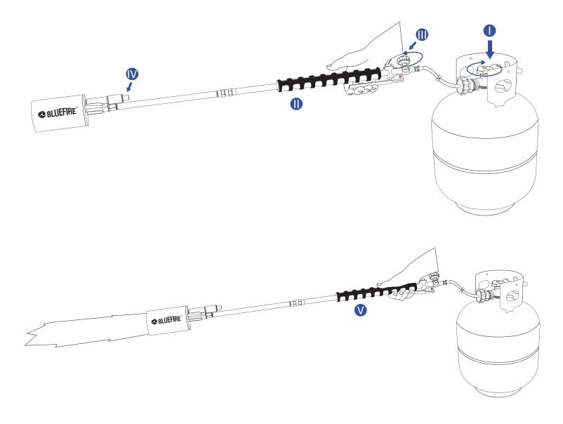
Step : To shut down, just turn off the main gas valve on the LP tank, let the flame naturally burns out all residue fuel gas inside the gas route.
