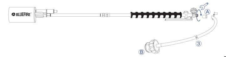
Step III: Connect hose end (B) to the LP tank adapter, tighten with the hand wheel. make sure the connection is secure and no leak occurs when turn on the main valve on the LP tank.
