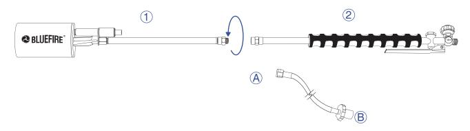
Step II: Unpack the hose, hose end (A) with female threading should be connect to the torch body, hose end (B) with hand wheel and male threading is for the LP tank. Connect (A) with Part (2), use wrench if necessary, DO NOT OVER-TIGHTEN!
