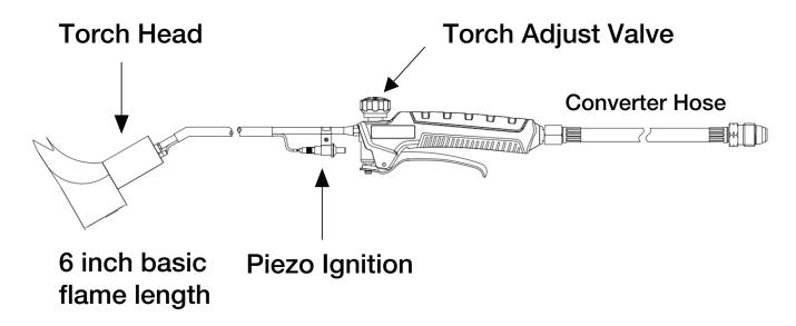
II.Keep the basic flame, when the Turbo Boost Trigger is depress, the flame become super flame.
