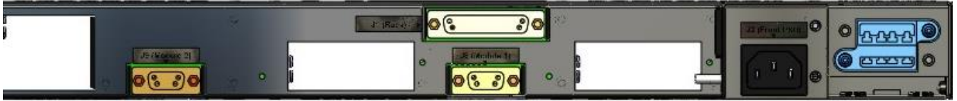
HRK1C View of interface connectors on the rear of the chassis (no modules fitted)
