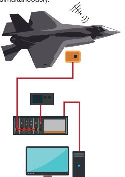
The controller also supports USB and Ethernet interfaces, allowing the system to be controlled from a PC.
