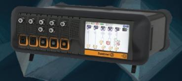
The 3U chassis is available in desktop and rack-mount format and accepts up to six single or dual receiver modules. Power and control distribution takes place via the chassis backplane. The unit also integrates battery charging.
