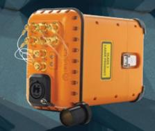
The compact remote transmitter is available with either one or eight inputs. It is double-screened for maximum shielding effectiveness and can be remotely controlled.
