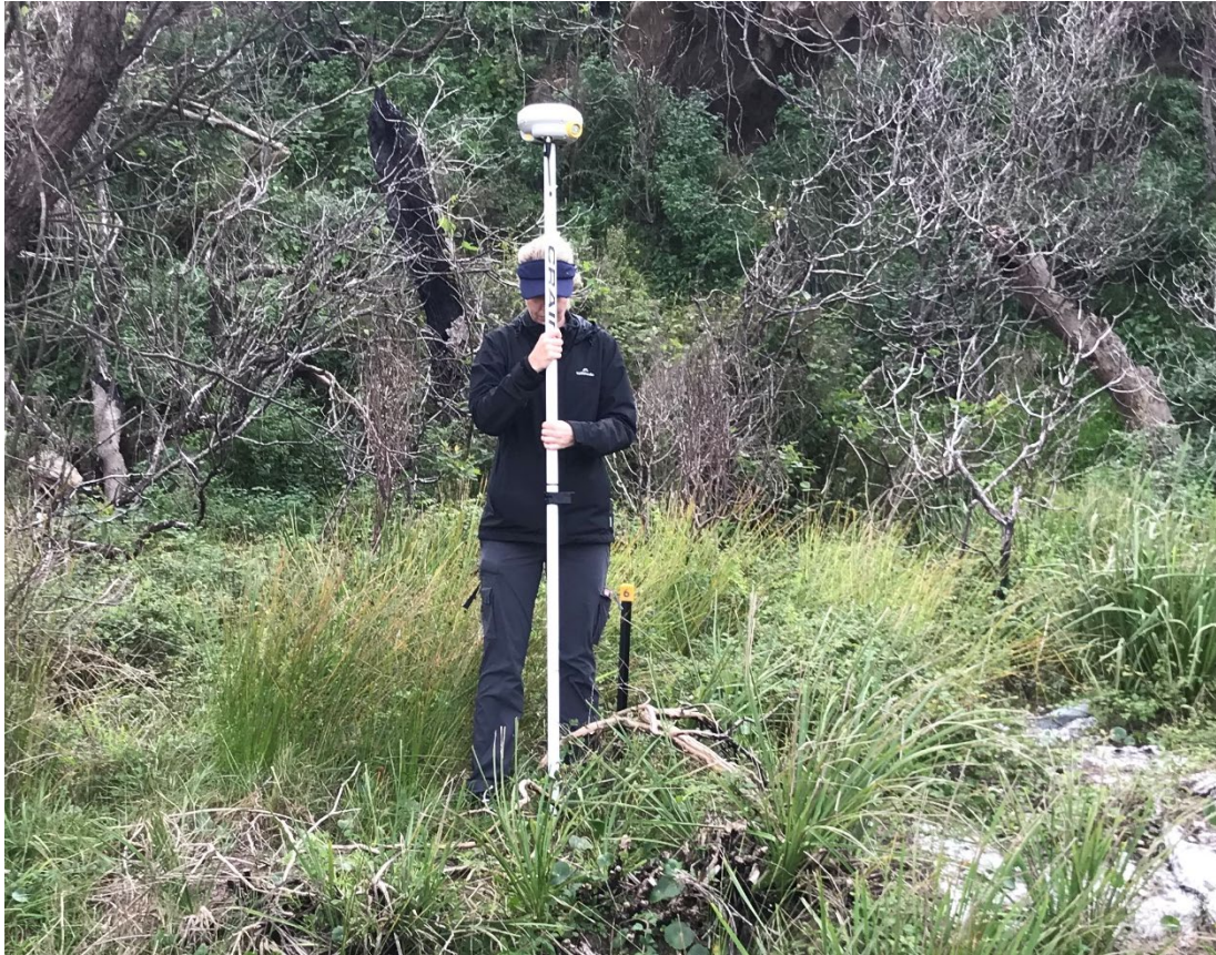
Figure 3. Surveying using the Trimble R4 RTK GPS and the temporary benchmark installed at the northern end of Rosedale Beach (metal fence post with numbered yellow safety cap).
