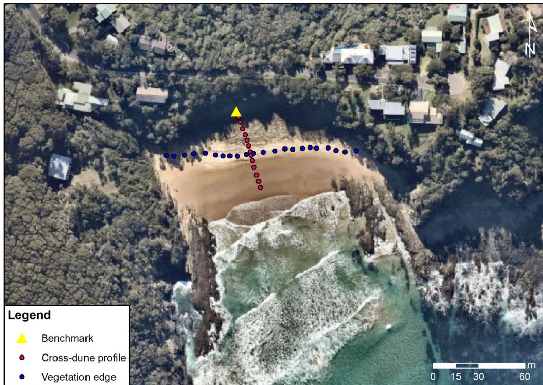
Figure 4. Example of survey data points collected at Nuns Beach on 9 April 2021 showing the temporary benchmark, the surveyed edge of the dune vegetation, and the cross-dune profile. Imagery source: nearmap (2019).
