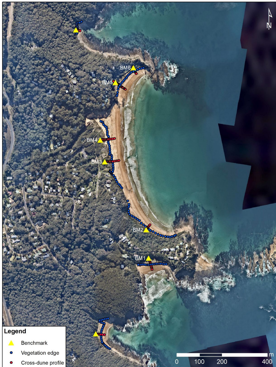
Figure 5. All survey data collected during the two days of in-situ data collection. Temporary benchmarks that were installed are labelled with "BM" and the benchmark number. Imagery source: nearmap (2019).
