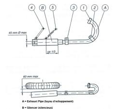
The exhaust pipe will be secured at a minimum of three points: to the engine head at one point (#1) and the frame at two points (#2 and #3).
