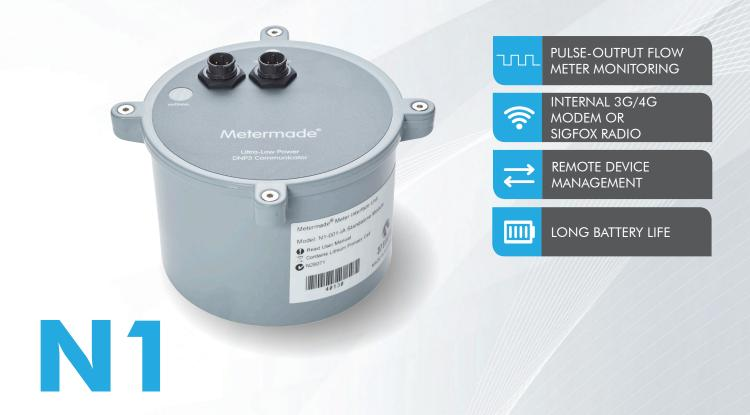
The Metermade® N1 Meter Interface Unit (MIU) is an ultra-low power device, designed to operate in the field for up to ten years on a single set of batteries (based on one report per day). It's housing meets the IP68 rating, permitting direct installation onto a flow meter and is capable of surviving submersion to a depth of four metres for four days.
