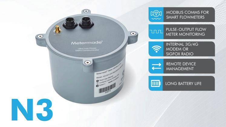
The Metermade® N3 Meter Interface Unit (MIU) is an ultra-low power device, designed to operate in the field for up to 5-10 years on a single set of batteries (based on one report per day). It's housing meets the IP68 rating, permitting direct installation onto a flow meter and is capable of surviving submersion to a depth of four metres for four days.
