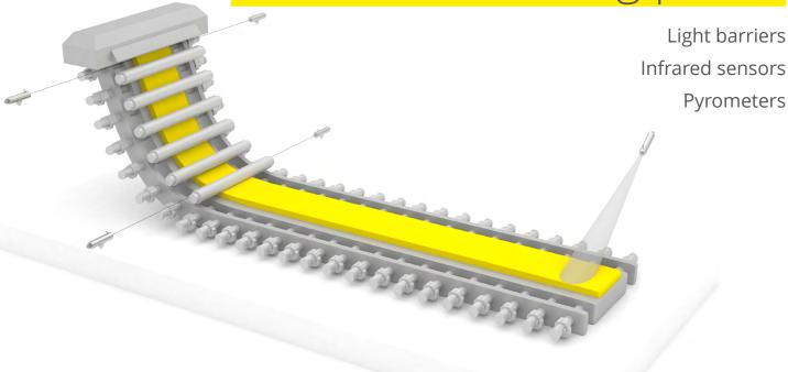
Continuous casting lines for slabs, blocks and billets continuously deliver semi-finished products for further processing in the rolling train. Proxitron light barriers and Piros infrared sensors are ideal for material recognition and monitoring in the area of the cut-to-length machine, and for the dummy bar detection. Pyrometers allow for accurate non-contact temperature measurement on materials up to 2500 °C.
