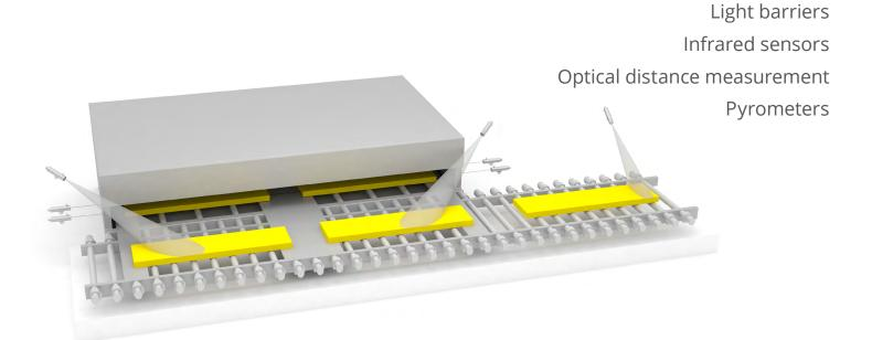
After the semi-finished material - e.g. a block - had been heated to the rolling temperature in a walking beam furnace, it is rolled to a defined measurement in the blooming train. In this area Proxitron infrared sensors or light barriers in the compact version or with fibre optic cable and separate optics suitable for ambient temperature up to 600 °C can be used for material tracking.
