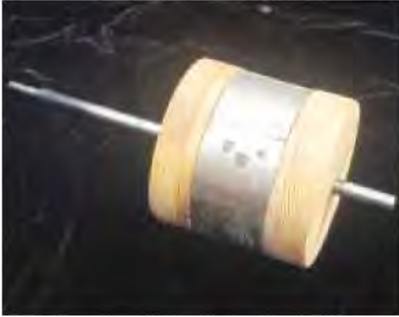
The wooden armature holds eight NdFeB (neodymium-iron-boron) magnets arranged in alternating polarity around its perimeter.
