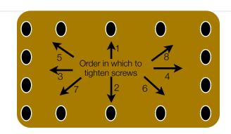
\*DO NOT USE A DRILL OR POWER SCREWDRIVER. DO NOT OVER TIGHTEN SCREWS\*
