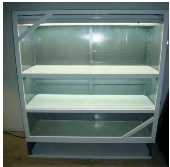
Figure 6: Grow chamber assembled and test run for a few days to make sure lighting works and there are no leaks in bottom or sides.
