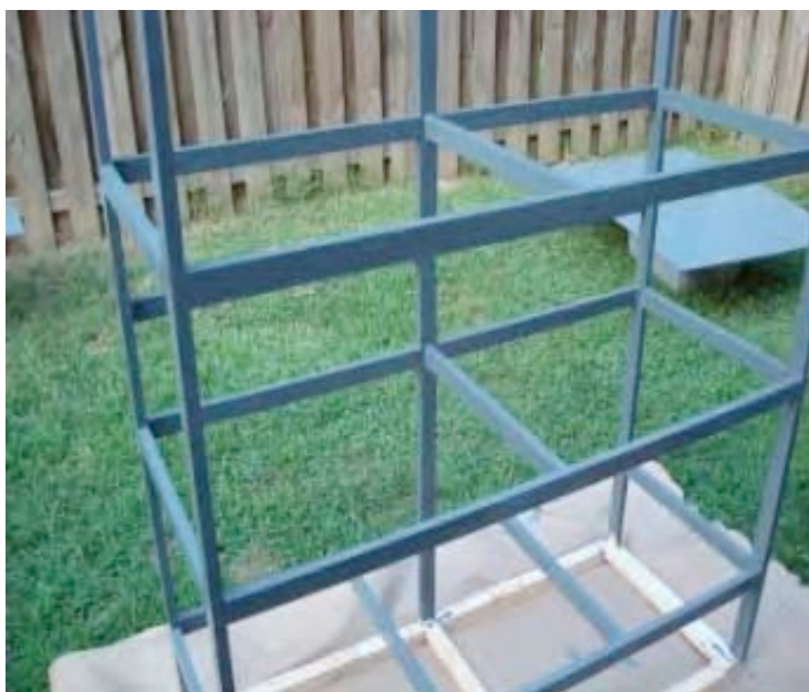
Figure 2: Frame coated with gray epoxy paint.
