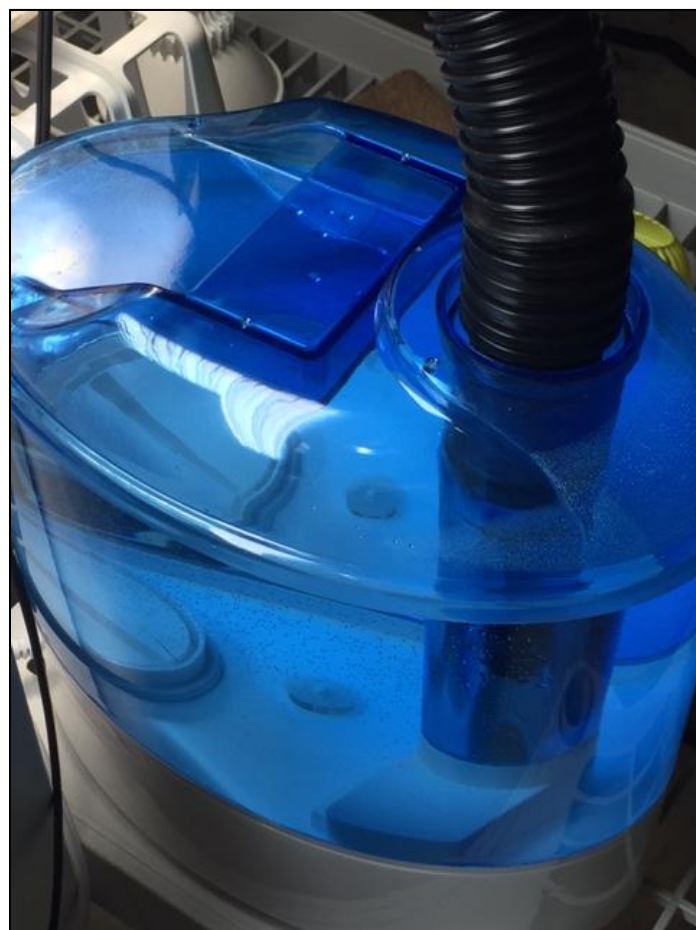
Humidifier which pumps in the humid fog
