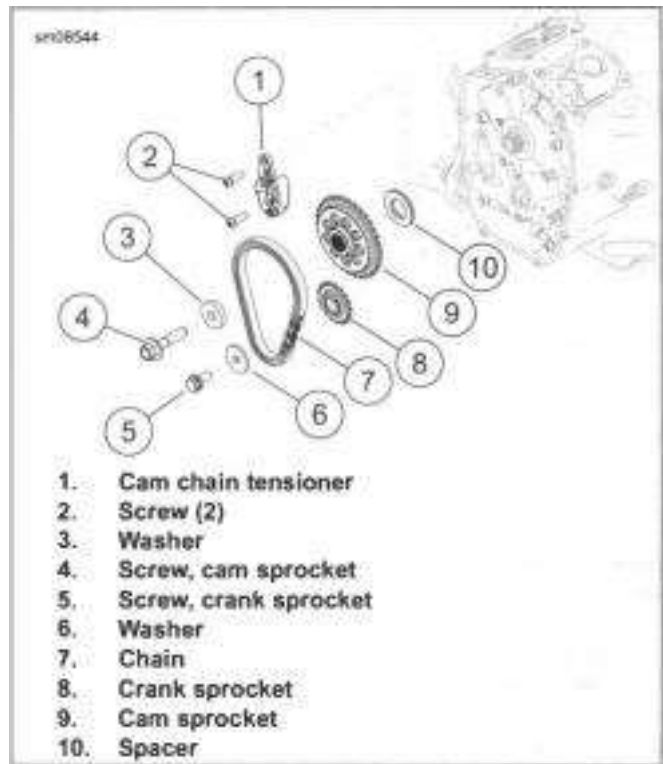
Figure 4-51. Camshaft Drive
