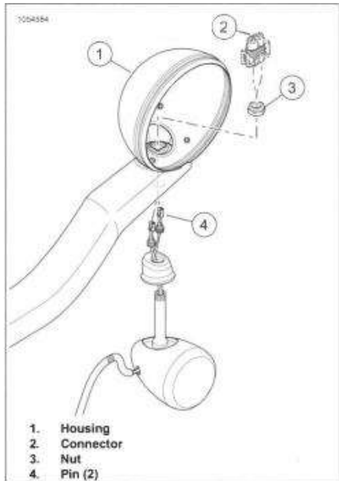
Figure 7-69. Auxiliary Lamp Housing with Incandescent Signal
