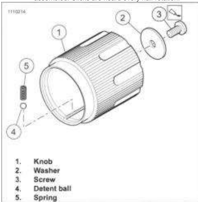
Figure 3-94. Rear Shock Adjuster Knob
