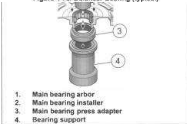
Figure 4-72. Install Left Main Bearing
