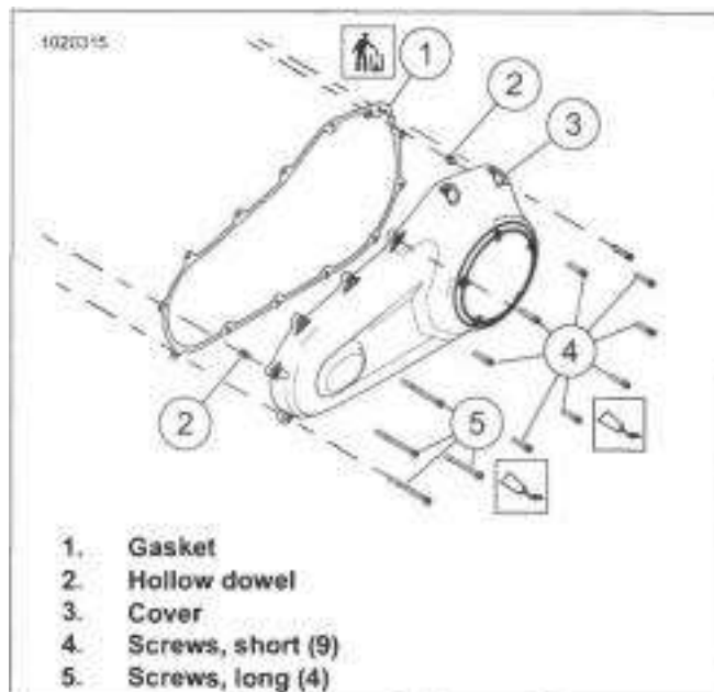
Figure 5-11. Primary Chaincase Cover
