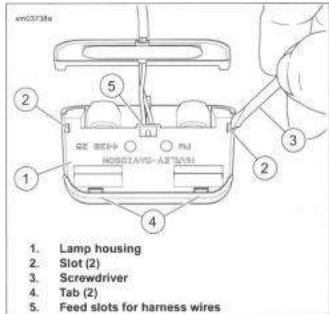
Figure 7-107. Removing License Plate Lamp Housing Cover
