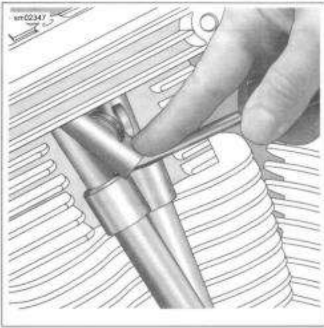
Figure 4-27. Install Spring Cap Retainers
