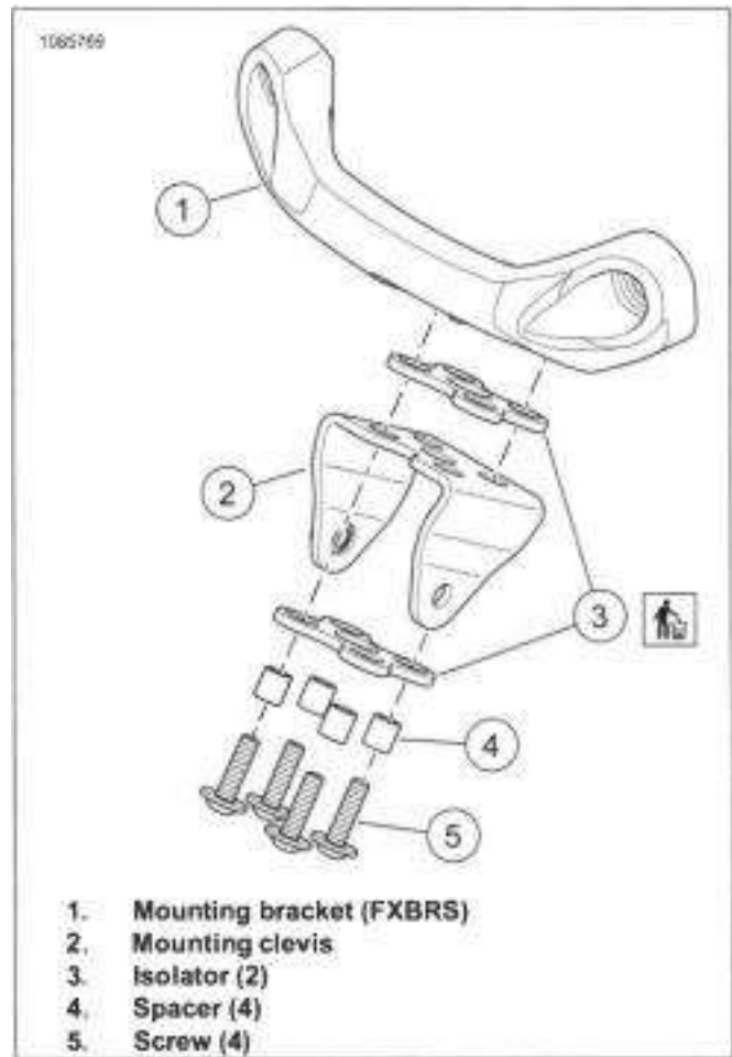
Figure 7-53. Oblong Headlamp Mounting Bracket (Typical)
