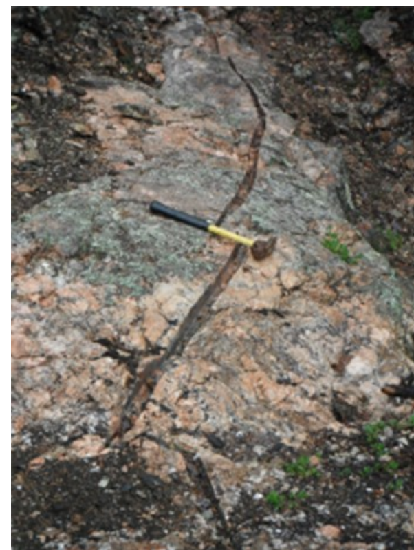
Channel Sample from Pegmatite dyke at Zoro Property
