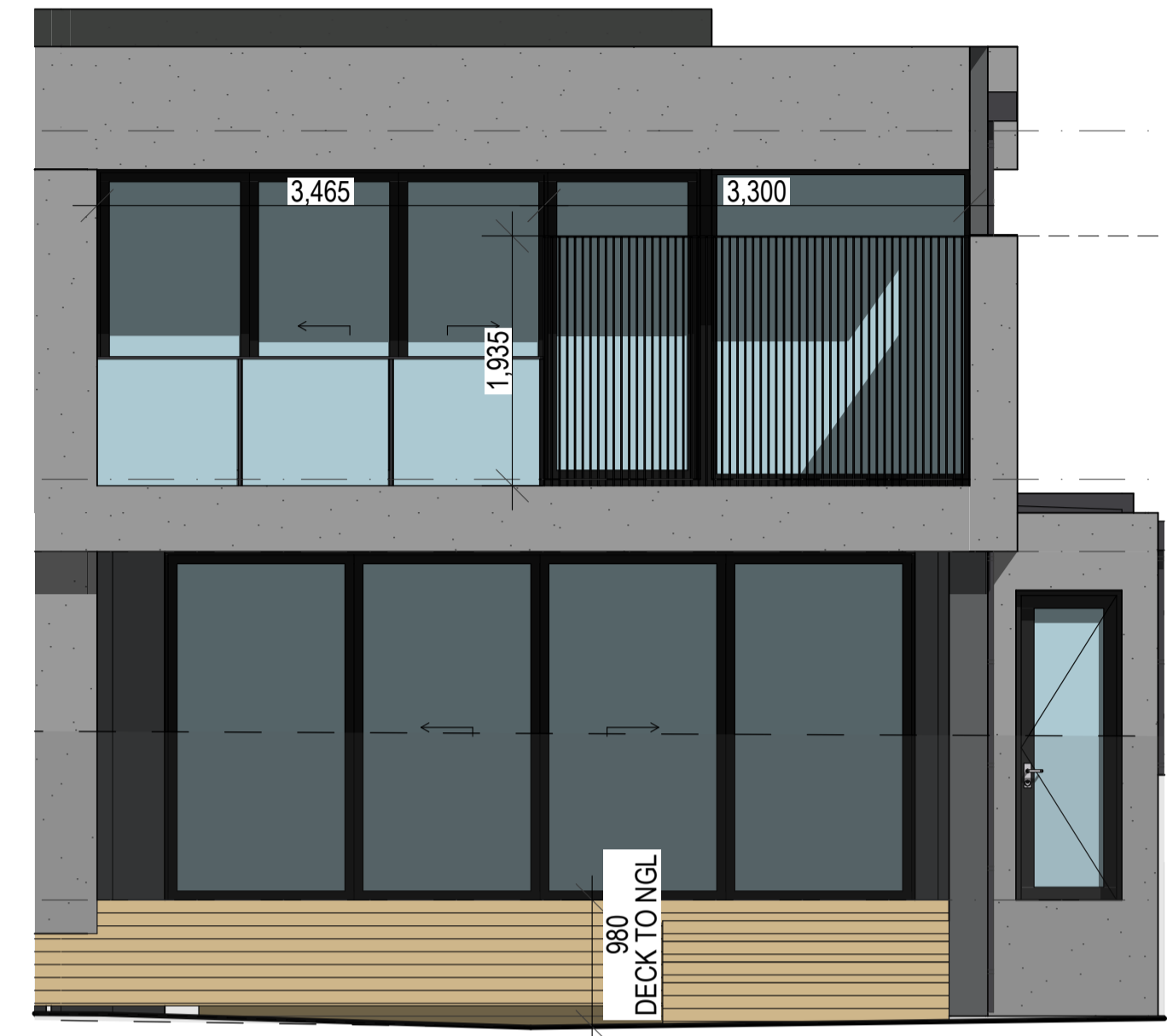
BALCONY BALUSTRADE - ELEVATION DETAIL SCALE 1:50
