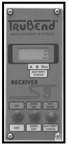
Turn the receiver on. Three bars will appear above RCV indicating that the battery condition is good.
