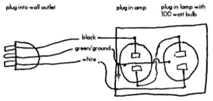
If you don't have one, build a simple current limiter out of a three-prong extension chord, a lamp, and a 100-watt lightbulb. (figure C) This project is quite simple, BUT IT DEALS WITH LETHAL **VOLTAGESI DO NOT TOUCH THE BARE WIRES, AND INSULATE EVERYTHING BEFORE YOU PLUG IT IN!** The idea is to put the bulb in series with the amp, so that all the current must first go through the lightbulb before it goes through the amp. This way, the bulb will not glow until the
