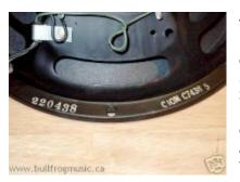
The speaker reads C10N C7438 5 on the right: which describes the model and its construction. But what about the 6-digit code 220438 to the left? That's the code that reveals the manufacturer as Jensen and the production date as the 38th week of 1964.
