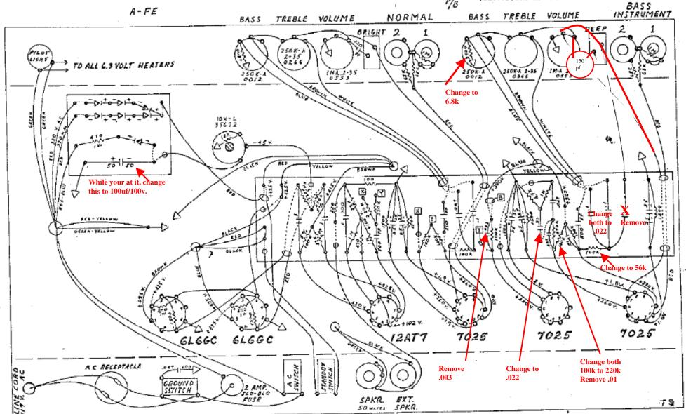
NOTE-ALL RESISTORS 1/2 WATT, 10 % TOLERANCE, IF NOT SPECIFIED
