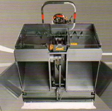
The proven snow elevator-chain-paddle system moves the scrapings from the ice to the snow bin effortlessly. The wide rear-access doors on the OLYMPIA™ 250's snow bin allows for ease of dumping.
