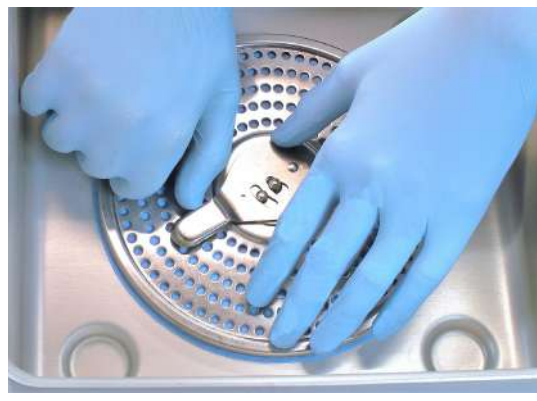
35 Rigid sterilization container filter placement
