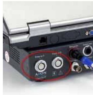
Figure 12: Preamp A (left) and Preamp B ports on Controller
