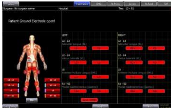
Figure 6: Electrode screen with open Patient Ground
