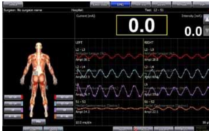
Figure 8: EMG test screen with 60Hz interference
