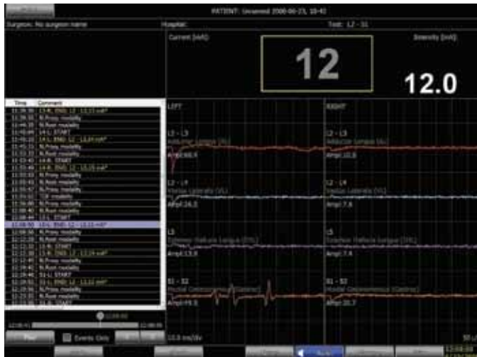
Figure 10: Stimulus artifact in the Left L2 – L3 channel causing false response (note the response begins at the start of the sweep and has a simple uniphasic shape)
