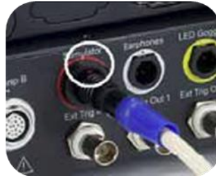
Figure 1: Align dots to connect Stimulator with Controller.
