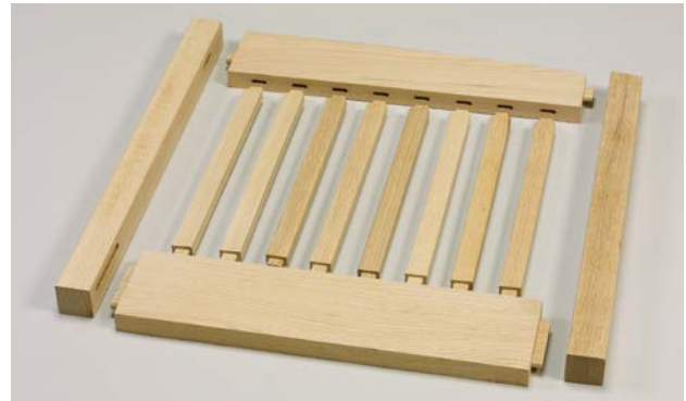
Mortise and tenon construction detail
