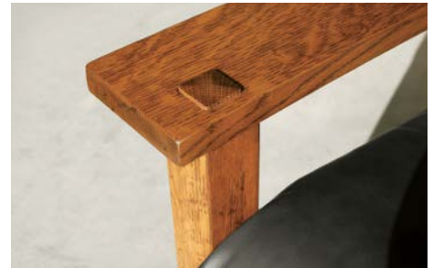
The classic look of mortise and tenon construction
