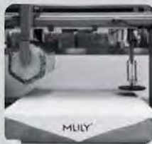
100,000 times mattress test Test number: QB/T1962.2
