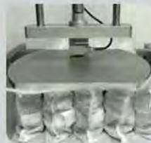
80,000 times spring test
