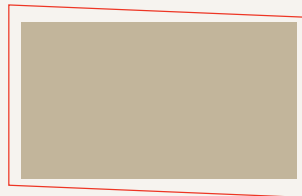
POOR BASE POSITIONING (CORNERS NOT AT RIGHT ANGLES)
