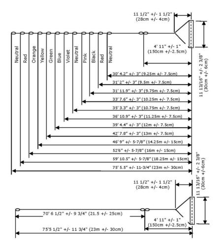
Note: For tournament-supplied handle sections, the bridle length shall be  $150 \text{ cm} \pm 2.5 \text{ cm} (4'11'' 1'')$  and the length of the handle shall be  $30 \text{ cm} \pm 6 \text{ cm} (11-13/16'' \pm 2-3/8'')$  (see diagram). For skier-supplied handles the tolerance on the bridle length is  $\pm 2.5 \text{ cm}/-10 \text{ cm} (\pm 1'')$ . (Return to Index)
