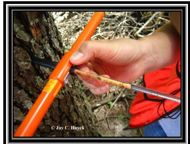
An increment core extracted from a black cherry tree using a Suunto™ increment borer.
