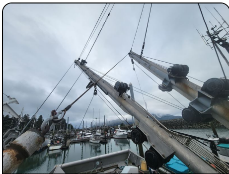
Photo 2: Twin main booms (tender vessel rig)
