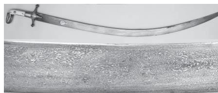
Figure 3: An Arab style saif, early 20th century, mounted with an earlier Persian shamshir blade. The 'watered steel' pattern is typical and reflects a dendritic pattern distorted by forging. (Photo credit: Lee A. Jones.)
