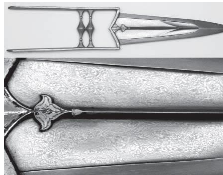
Figure 2: Indian katar (jamadhar) of the 18th century with an exceptional wootz pattern; the best work features bold patterns with high contrast such as seen in this example. This wavy pattern of shiny and dark steel is made up of networks showing different metallographic structures (specifically globular cementite in a matrix of pearlite) and extends through the full thickness of the blade, appearing similar at any angle of intersection with the varied surfaces. Foci of a cast crystalline dendritic structure appear to have been retained in this blade indicating very restrained forging and stock removal to create the high central rib and other topographic features. (Photo credit: Lee A. Jones.)
