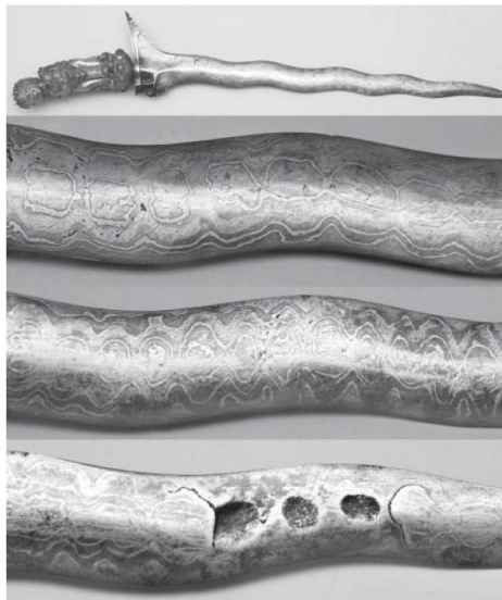
Figure 2: Another Balinese keris, probably later 19th century, with a blade pamor formed by relatively coarsely laminated contrasting steel alloys, the lighter steel containing nickel for sharp contrast. Aesthetics in Bali lean more towards a polished blade, such as this example, than the etched surface currently favored in Java. In this example, the layers are again oriented parallel to the plane of the blade (mlumah) and have been intentionally distorted by shallow holes or punch work prior to the surface being reforged flat to create the pattern. Repeated cleaning and polishing have disclosed a once hidden zone of failed weld adherence (cold shut) between two layers and depressions are now left where the surface has fallen away over the defect. Adjacent cracks foretell further surface losses should the blade be polished again. (Photo credit: Lee A. Jones.)
