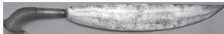
Figure 6: The wide blade of this early 20th century Philippine barong shows several bands of alternating contrasting patination which converge at the tip and towards the hilt where the blade narrows. This evidence of piled construction is barely visible on the opposite blade face.
