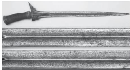
Figure 1: Balinese keris, probably earlier 20th century, with a blade pamor formed by coarsely laminated contrasting steel alloys. In this case, the layers are oriented parallel to the plane of the blade (mlumah) and have been intentionally manipulated to intersect with the ultimate etched blade surface to create the pattern. (Photo credit Lee A. Jones.)
