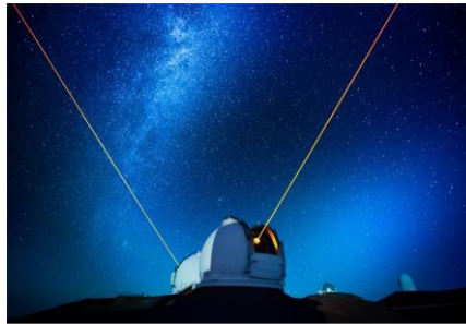
Figure 4: Twin 10-meter Keck telescopes. Note: lasers are used to control adaptive optics to counter atmospheric turbulence. https://www.keckobservatory.org/about/keck-observatory/
