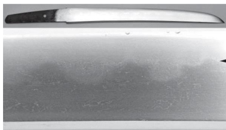
Figure 4: Nioi appearing as a misty line along the hamon in a 17th Century Japanese tanto (dagger) blade. As the hamon is a boundary formed at the time of quenching, the term 'temper line' is a misnomer. (Photo credit: Lee A. Jones.)
