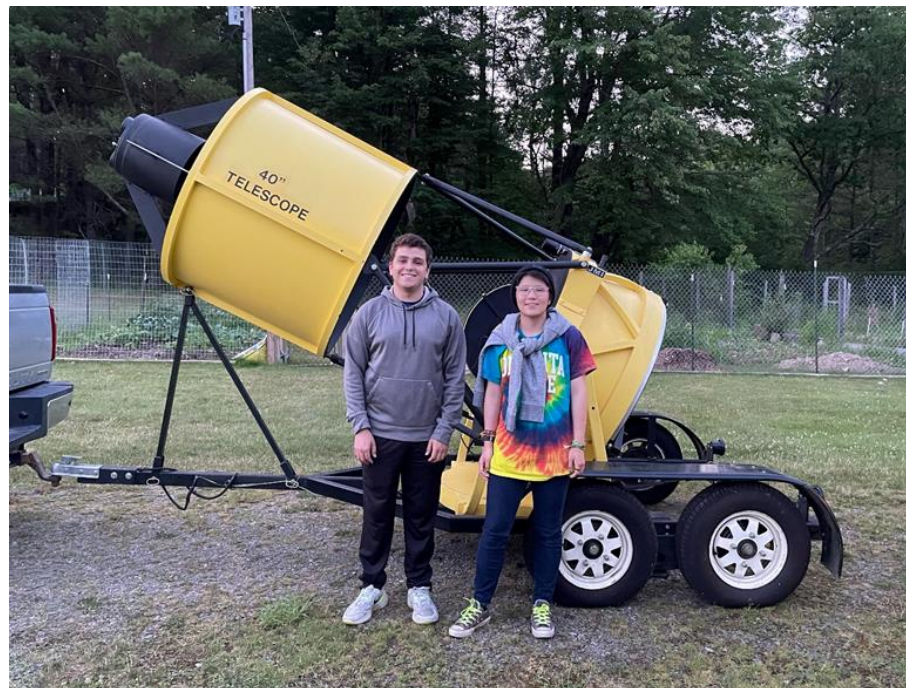
Figure 1: Dr. Rapson's Students Joshua and Hadley Chan in front of SUNY Oneonta's JMI 40" Alt-Azimuth Folded Newtonian Mounted on a Trailer.
