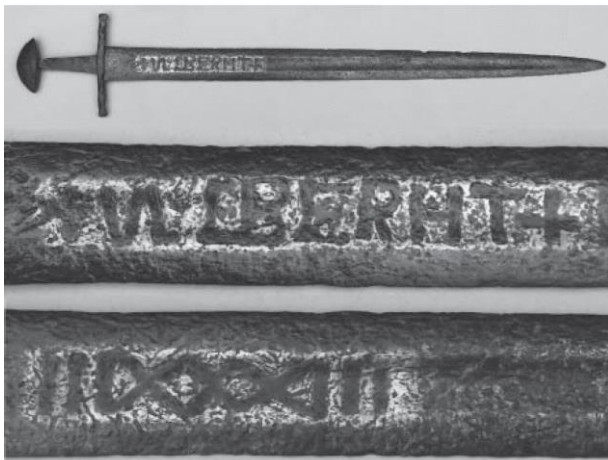
Figure 4: A European sword of the mid to late Viking Age, mid 10th to early 11th century, bearing a variant of the +ULFBERHT+ inscription on one face of the forte and a geometric pattern on the opposite face. The inlay is composed of twisted rods made from stacked steels of varying composition likely forged into grooves in the face of the blade and then dressed flat. Though contemporary with the Vikings, the brazil nut pommel suggests mounting nearer the origin of the blade, speculated to have been in what is now Germany. The steel surrounding the inscription has been brightened by polishing to increase contrast.
