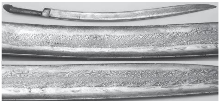
Figure 2: A yataghan, probably 18th century, characteristic of Turkey and the areas within the influence of the Ottoman Empire. In addition to laminated (layered) steel on its edge and back, the blade shows three bands of twist core patterned steel running the length of the blade. This pattern, created from a twisted rod incorporated into the blade for each band, repeats itself along each band with slight changes as curved patterns merge into a zone where the appearance is more that of diagonal lines.
