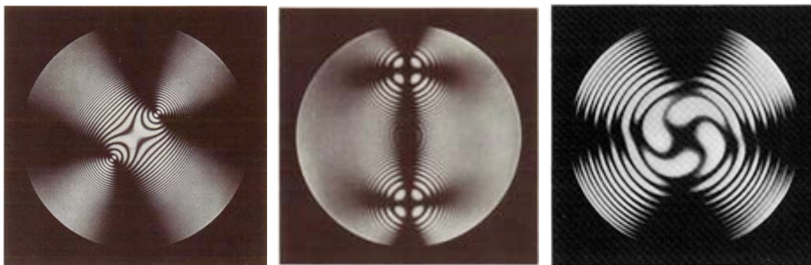
Interference figures photographed in monochromatic sodium light: Left, biaxial figure; center, twinned crystal; right, Airy's spiral. From Hans Hauswaldt's "Interferenze-Erscheinungen", 1902; this was the first of a remarkable 3-volume series, published from 1902 – 1908.
