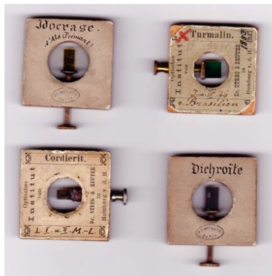
A selection of rotating mounts; these were intended to demonstrate pleochroism while turning the brass handle.
