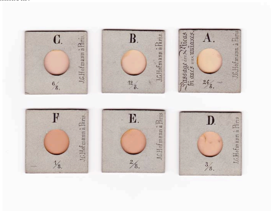
A set of Nörrenberg crossed mica plates to demonstrate the formation of a pseudo-uniaxial character in 3-T micas.
