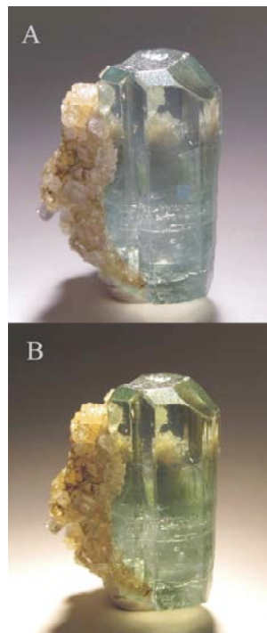
Figure 1. Apatite color change due to incident light. A) Blue in incandescent light, B) green in halogen light.
