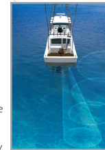
Without a fairing, the beam is angled improperly.
