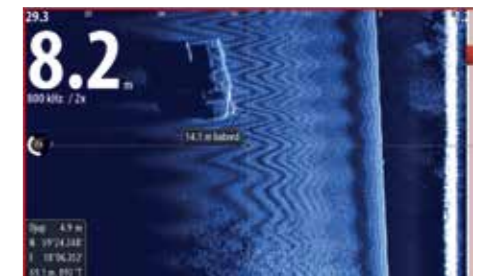
Underwater truck wreck (showing the left hand side of a SideScan view)
