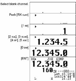
The set frequency can be cleared when [RX clas] is pushed while setting.
