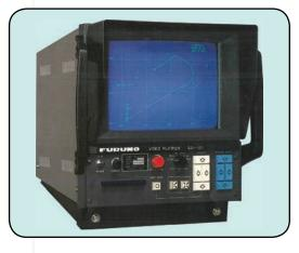
The world's first video Plotter, the Furuno GD-101, displayed Loran position and ship's Track on a simple vector grid.
