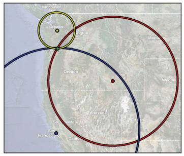
Figure 1 - Example of GPS Trilateration
