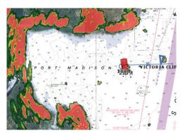
Example of Raster Chart with Radar Overlay and Satellite Photo Fusion
