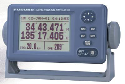
The GP-37 is an advanced GPS navigator designed for coastal ships, fishing boats and pleasure craft. It is equipped with a WAAS receiver and a DGPS receiver as standard supply. The powerful processor performs high-speed processing, position fixing and augmentation. It utilizes both WAAS and differential radio beacon correction methods.
