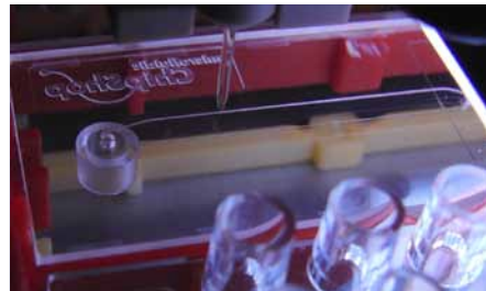
Fig. 564: instrument TWO-200 spotting in microfluidic devices DNA-Array embedded in a microfluidic channel
