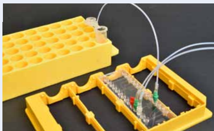
Fig. 678: Complete experimental setup with the exit port of the droplet generator connected to a collection vessel
