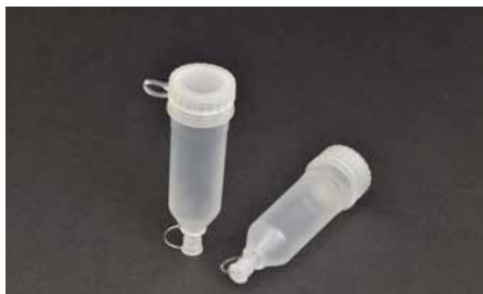
Fig. 493: Sampling vessel a total volume of 6.5 ml
