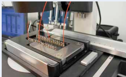
Fig 689: Lab-on-a-Chip Cell Culture Incubator – LOC CCI 1 with embedded chip and capillaries for the connection of pumps
