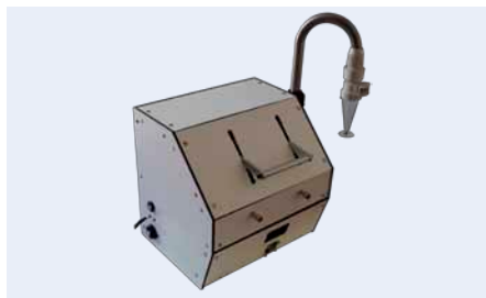
Fig. 767: Breadboard system: Electrochemical immunoassay system for air sample analysis, FP7 project Multisense Chip, No. 261810
