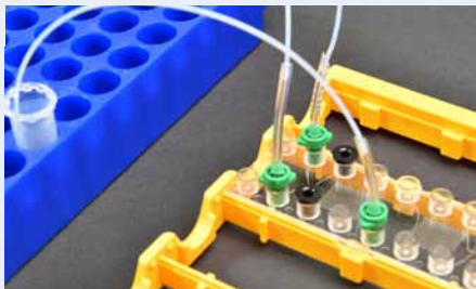
Fig. 663: Close unused fluid ports on chip with red Luer plugs
