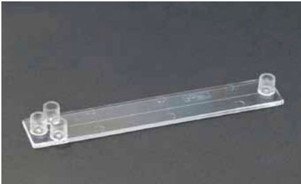
Fig. 58: Cross-shaped channel chip with Luer interfaces
