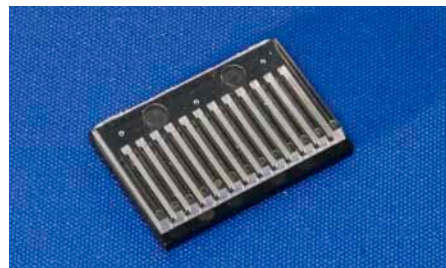
Fig. 764: Microfluidic chip realized for CARE-MAN - Health-CARE by biosensor Measurement and Networking, FP 6, NMP4-CT-2006-017333
