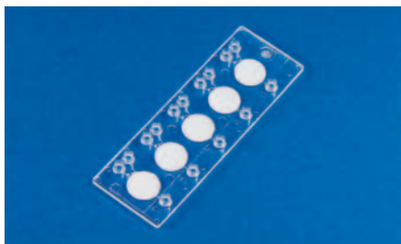
Fig. 737: Hybrid chip consisting of polymer and filters for plasma generation
