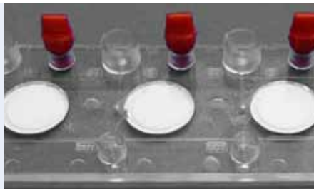
Fig 684: Membrane chip Fl. 200 with Mini Luer plugs
