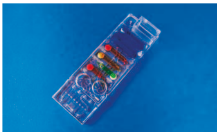
Fig. 739: Hybrid chip for immunoassays with electrochemical detection, realized within the EU-FP6 project "SmartHEALTH", No. 016817
