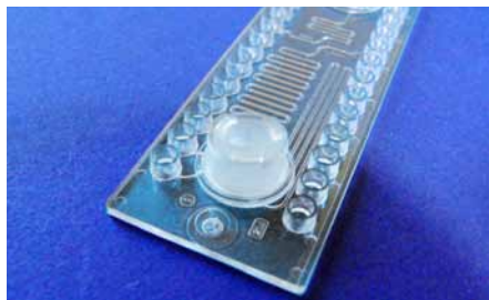
Fig. 750: Fluidic chip with rotary valve
