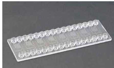
Fig. 218: Droplet generator – Similar chip layout for both Fluidic 440 and Fluidic 947
