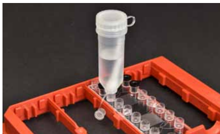
Fig. 494: Sampling vessel prefilled with buffer and inserted swab
