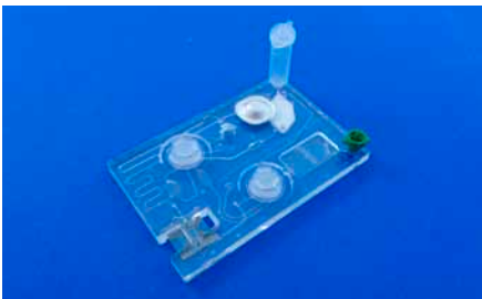
Fig. 789: Photonic biosensing chip for microRNA-based early diagnosis of diseases - Fluidic 866 Horizon 2020 project, Grant agreement no: 644242
