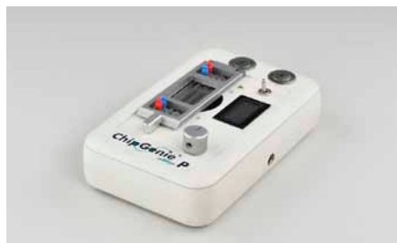
Fig. 542: ChipGenie® edition P instrument with inserted chip
