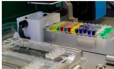
Fig. 181: 65-well chip used as source plate in spotter
