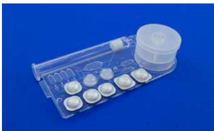
Fig. 784: Immunoassay-Chip for mycotoxine analysis, BMBF-Project Kombispec, FKZ 13N13757
