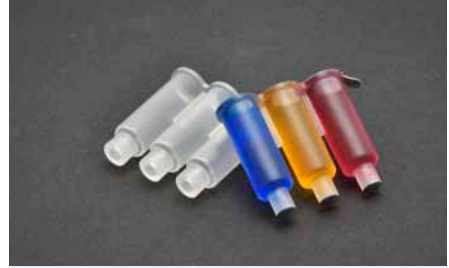
Fig. 470: Filled tanks sealed with alumina foil
