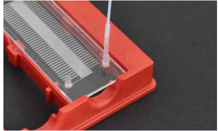
Fig. 502: PTFE tubing interconnected via silicone sleeve to the olive interface of a microfluidic device
