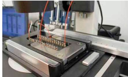
Fig. 552: Lab-on-a-Chip Cell Culture Incubator – LOC CCI 1 placed on a microscopy stage
