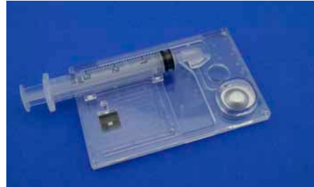
Fig. 772: Selective cell counting chip for hematology, BMBF project MrCyte, FKZ 13N12018
