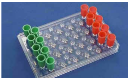
Fig. 781: Organ-on-chip device operated with hydrostatic fluid management, BMBF project HepaChip, FKZ 031A121D
