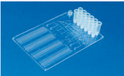
Fig. 747: Sample-in-result-out DNA-analysis chip with hybridisation zone for optoelectronic read-out, realized within the project Pathold Chip, A-102-RT-GC
