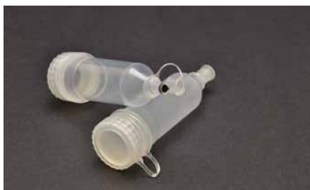
Fig. 495: Sampling vessel with pierceable septum
