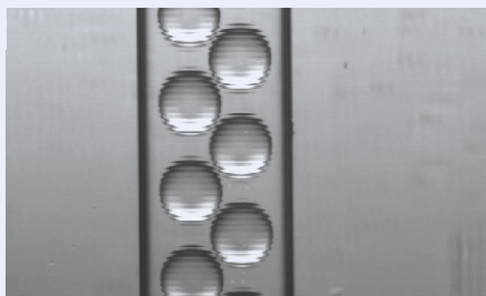
Fig. 679: Droplets generated on chip
