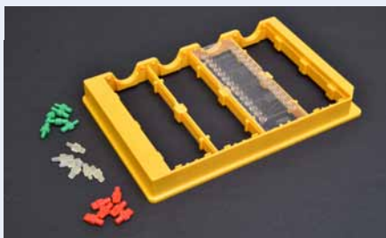
Fig. 674: Droplet generator Fluidic 285 placed in handling frame
