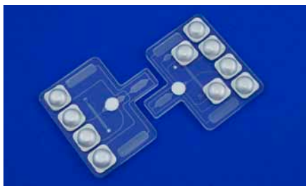
Fig. 783: Immunoassay-Chip, BMBF-Project HandyLoC, FKZ 13N13714
