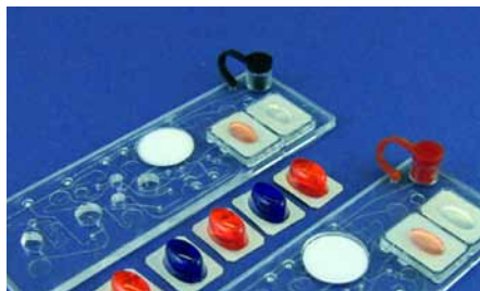
Fig. 752: Immunoassay chip with plasma generation unit and blister pouches
