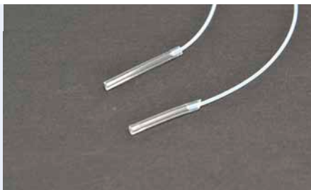
Fig. 667: Short pieces of silicone tubes connected with PTFE tube
