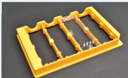
Fig. 666: Microfluidic chip with olive interfaces inserted in a microfluidic chip handling frame
