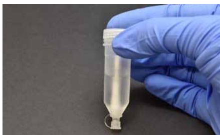
Fig. 496: Sampling vessel prefilled with buffer and inserted swab
