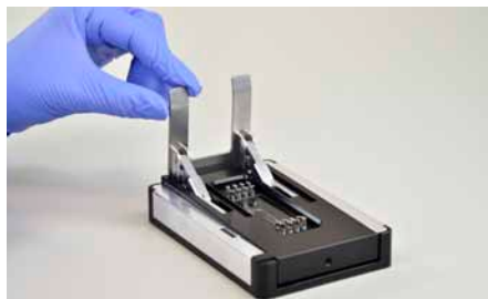
Fig. 398: Layout LOC HP/CCI 1 – Handling frame for chips in the format of a microscope slide
