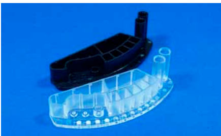
Fig. 763: Chip cuvette for frit-based immunoassays, realized within the BMBF project IFSA, FKZ 16SV5417
