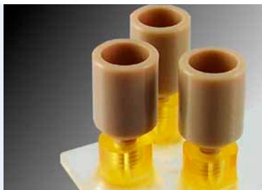
Fig. 446: Cross-shaped channel chip with three bonded port connectors and three chip reservoirs
