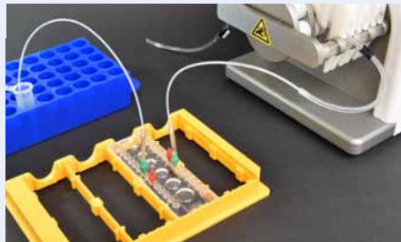
Fig. 653: Connection of the chip via the PTFE tube with the pump
