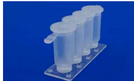
Fig. 788: Transwell membrane chip Fluidic 219 with tank Fluidic 235 as fluid reservoir, TAB project number 2013 FE 9021
