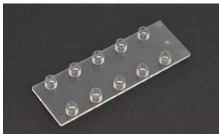
Fig. 712: Example of microscopy slide Luer platform with ten Luer interfaces
