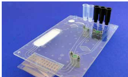
Fig. 754: Serology test chip for the detection of coeliac disease, realized within the FP 7 project "CD-Medics", No.216031
