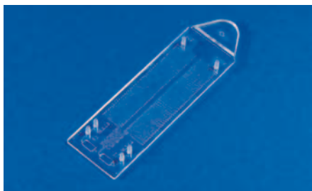
Fig. 738: Continuous-flow PCR chip, chip, realized within the BMBF-Project "ChipFlussPCR", FKZ 13N9556
