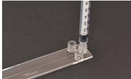
Fig. 59: Cross-shaped channel chip with female Luer interface and a syringe as male counterpart
