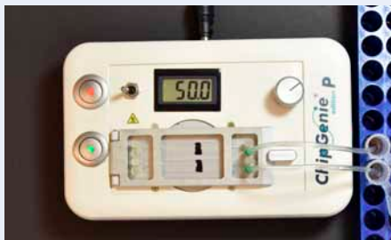
Fig. 683: ChipGenie® edition P instrument with washing buffer inside the rhombic chamber.
