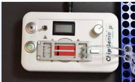
Fig. 682: ChipGenie® edition P instrument with a blood sample inside the rhombic chamber. The magnetic beads, migrating through the chambers, are visible as black bars.
