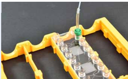
Fig. 661: Insertion of the Luer with tubings in fluid entrance of the chip
