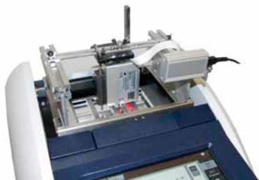
Fig. 632: Implementation of low-volume real-time PCR on chip – Chip on breadboard instrument
