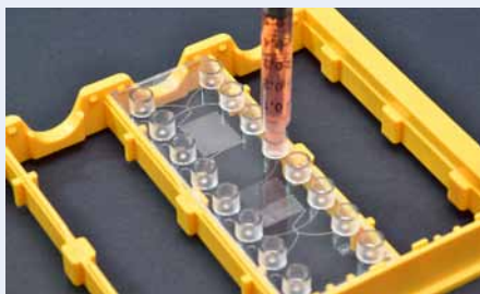
Fig. 655: Microfluidic chip with Luer interfaces filled with a standard syringe
