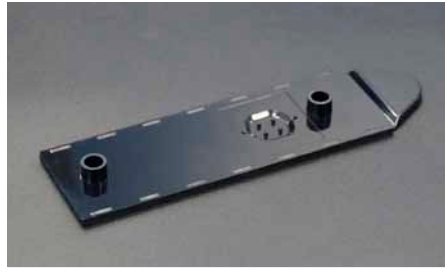
Fig. 130: Straight channel chip – black
