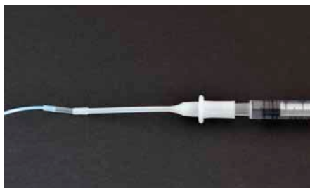
Fig. 425: Syringe adapter interconnecting a 1 ml syringe and silicone sleeve of microfluidic tubing
