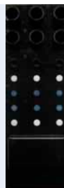
Fig. 636: Implementation of frit-based immunoassay on chip – Target: Troponin, colorimetric detection: poly HRP (pHRP)/TMB (blue dye)
