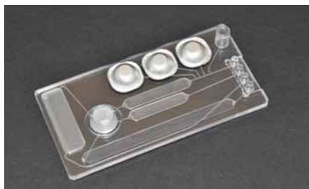
Fig. 487: DNA analysis chip with blister and integrated lateral flow strip
