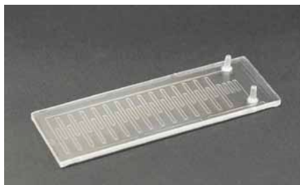
Fig. 534: 15-cycle continuous-flow PCR-chip
