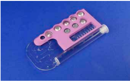
Fig. 785: Real-time PCR chip for B-agent detection, Horizon 2020 project, No. 700264
