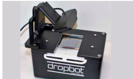
Fig. 556: DropBot instrument for manipulation and read-out
