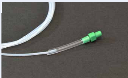
Fig. 649: Connection of Mini Luer fluid connector with mounted silicone sleeve with a PTFE tube
