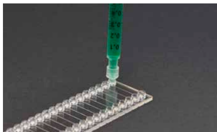
Fig. 427: Example of a Mini Luer to Luer adaptor in use with a straight channel chip
