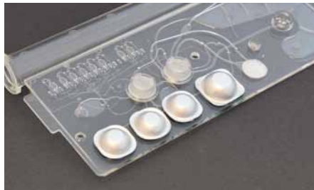
Fig. 452: Blister pouches of different volumes integrated in a complex microfluidic chip
