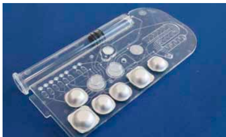
Fig. 779: Integrated microfluidic chip for the detection of viral pathogens in the food supply chain, FP7 project EDEN, No. 313077
