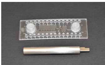
Fig. 313: Turning valve test chip with manual turning valve actuator
