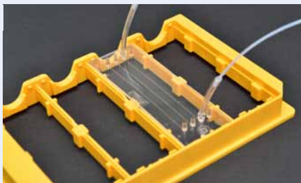
Fig. 668: Chip with olive interfaces connected with tubes
