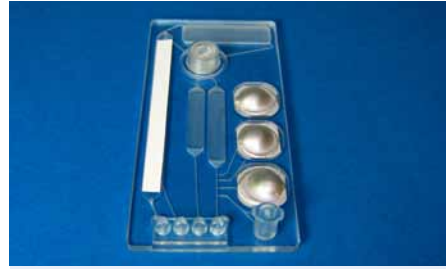
Fig. 758: Microfluidic chip with lateral flow strip based detection and implemented blister for liquid storage
