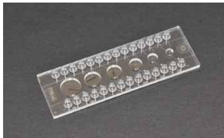
Fig. 168: Micro mixer with magnetic stir bars for active mixing
