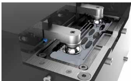
Fig. 543: Blisters of blister test chip being actuated by the ChipGenie® edition BD instrument
