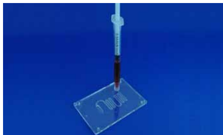
Fig. 755: Boyle-Mariotte PCR chip for ultrafast PCR, design: IMM, realized within the FP 7 project "CD-Medics", No. 216031
