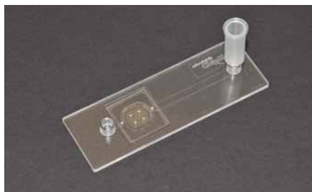
Fig. 466: 500 µl single tank mounted on Luer interface
