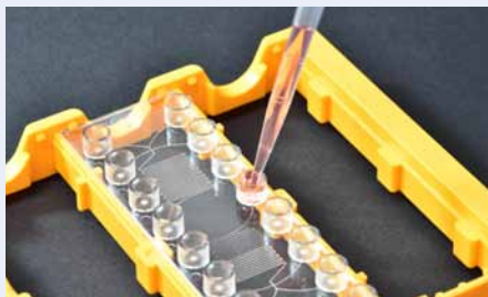
Fig. 656: Microfluidic chip with Luer interfaces filled with a pipette and interfaces used as reservoir
