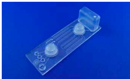
Fig. 756: Enzyme-assay development chip, realized within the FP 7 project Multisense Chip, No. 261810
