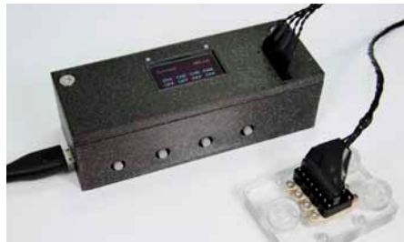
Fig. 603: Control system and connected valve manifold
