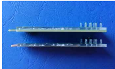
Fig. 748: Microfluidic chip coupled to conventional (top) and flex (bottom) PCBs, realized within the BMBF-project "Safels", FKZ 0315574C
