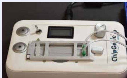
Fig 681: Chip inserted into ChipGenie® edition P instrument and installed connectors with silicone sleeve and PTFE tubing.
