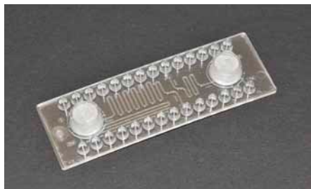
Fig. 497: Fluidic chip with embedded rotary valve
