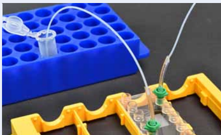
Fig. 662: Insertion of the Luer with tubings in fluid exit of the chip and connection of tube with sampling vessel
