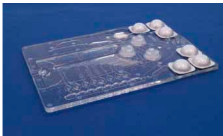
Fig. 777: Integrated microfluidic chip for the detection of bacterial pathogens, FP7 project Multisense Chip, No. 261810
