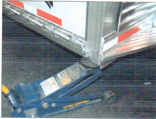
Jacking Point for Trailer
