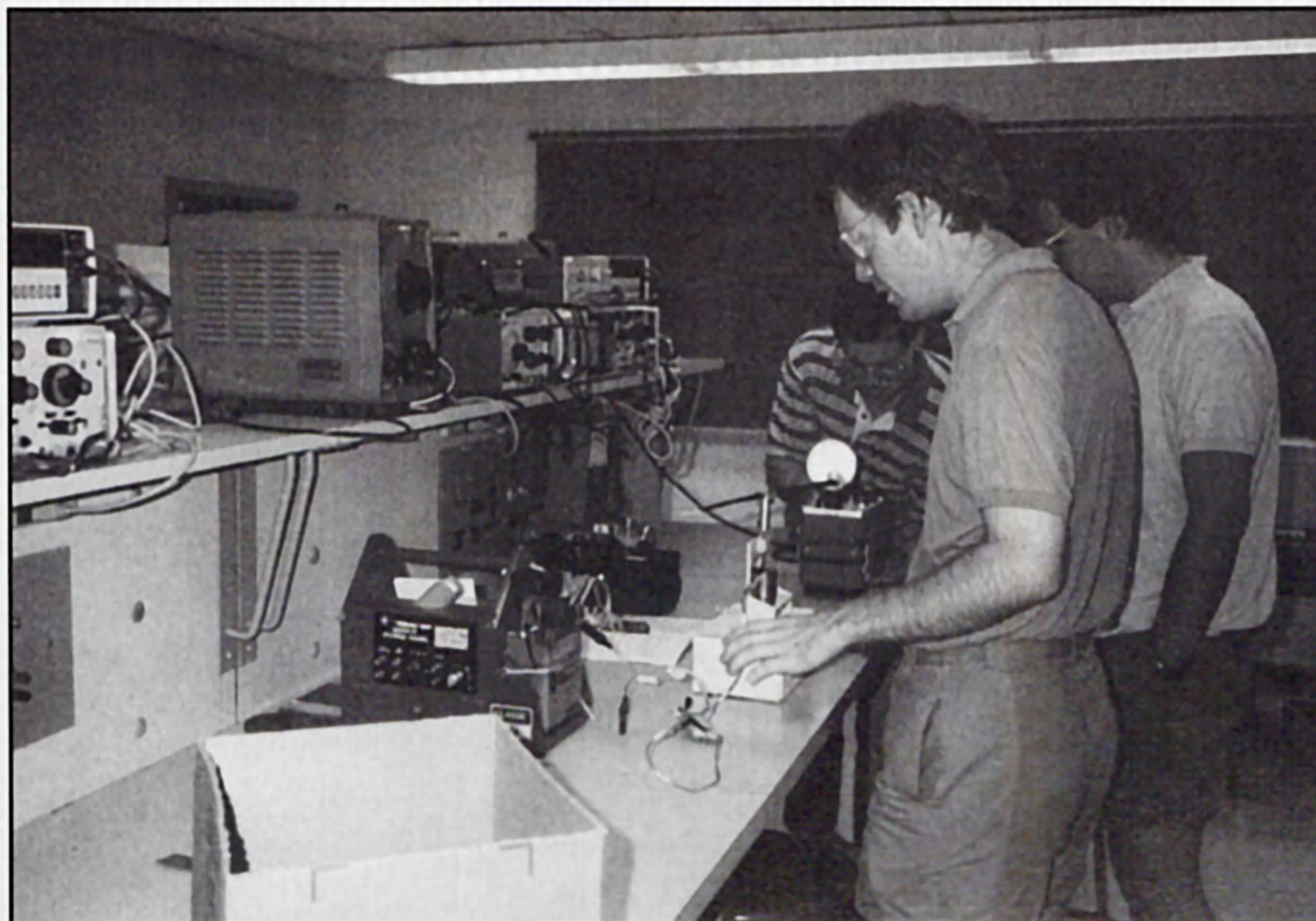
Left: The pennies in the box under the test stand rattled loudly at certain rotor speeds. Strobe tests in an electronics laboratory at Purdue University revealed that the soft basswood blades fluttered at high speed causing excessive vibration and drag. Right: Small amounts of aluminum melt easily with a propane torch. At 1300°F, molten aluminum will pour and splash as easily as water, so we were very careful and always wore appropriate safety gear.
