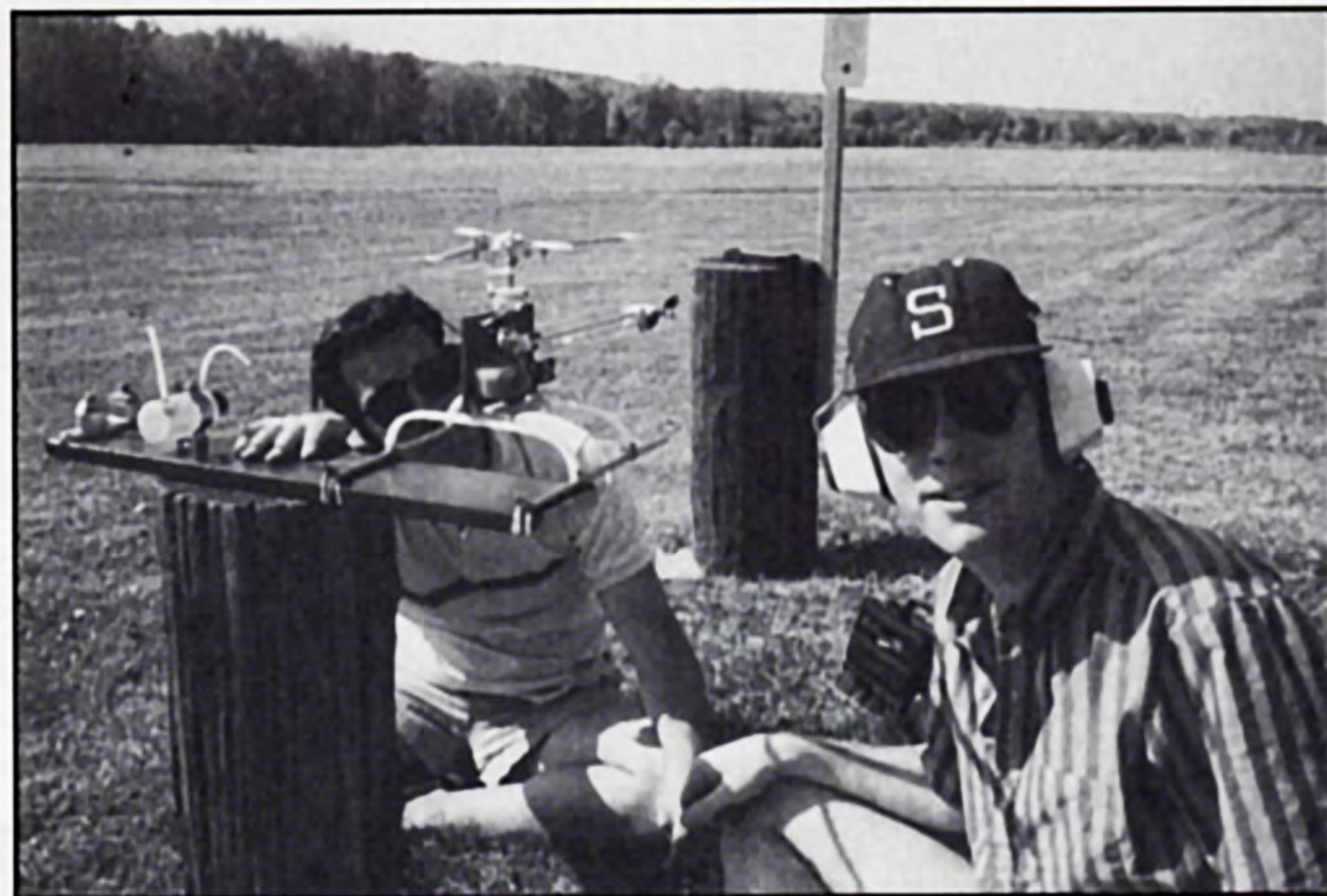
Left: This sophisticated experimental casting/sintering apparatus for making gear molds involved a propane torch, brownie pan lined with kitty litter, and tank of compressed nitrogen on our back patio. We always perform delicate experiments such as this outdoors at night under the most adverse weather conditions. Right: This Cox 049 powered test mechanism preceded Prototype I. The main rotor and tail rotor are fully functional and ready to be mounted to an airframe with radio.
