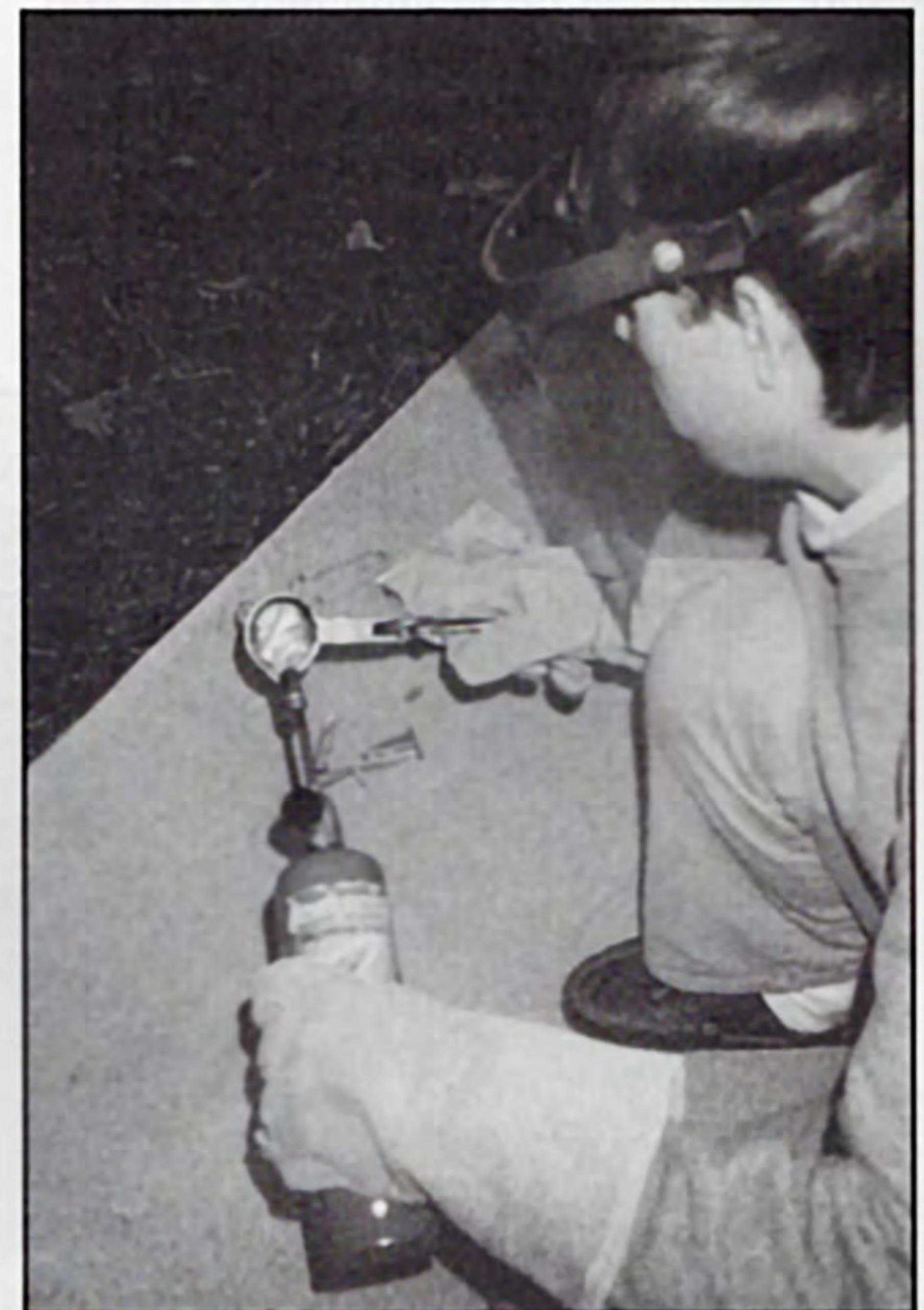
Left: The pennies in the box under the test stand rattled loudly at certain rotor speeds. Strobe tests in an electronics laboratory at Purdue University revealed that the soft basswood blades fluttered at high speed causing excessive vibration and drag. Right: Small amounts of aluminum melt easily with a propane torch. At 1300°F, molten aluminum will pour and splash as easily as water, so we were very careful and always wore appropriate safety gear.
