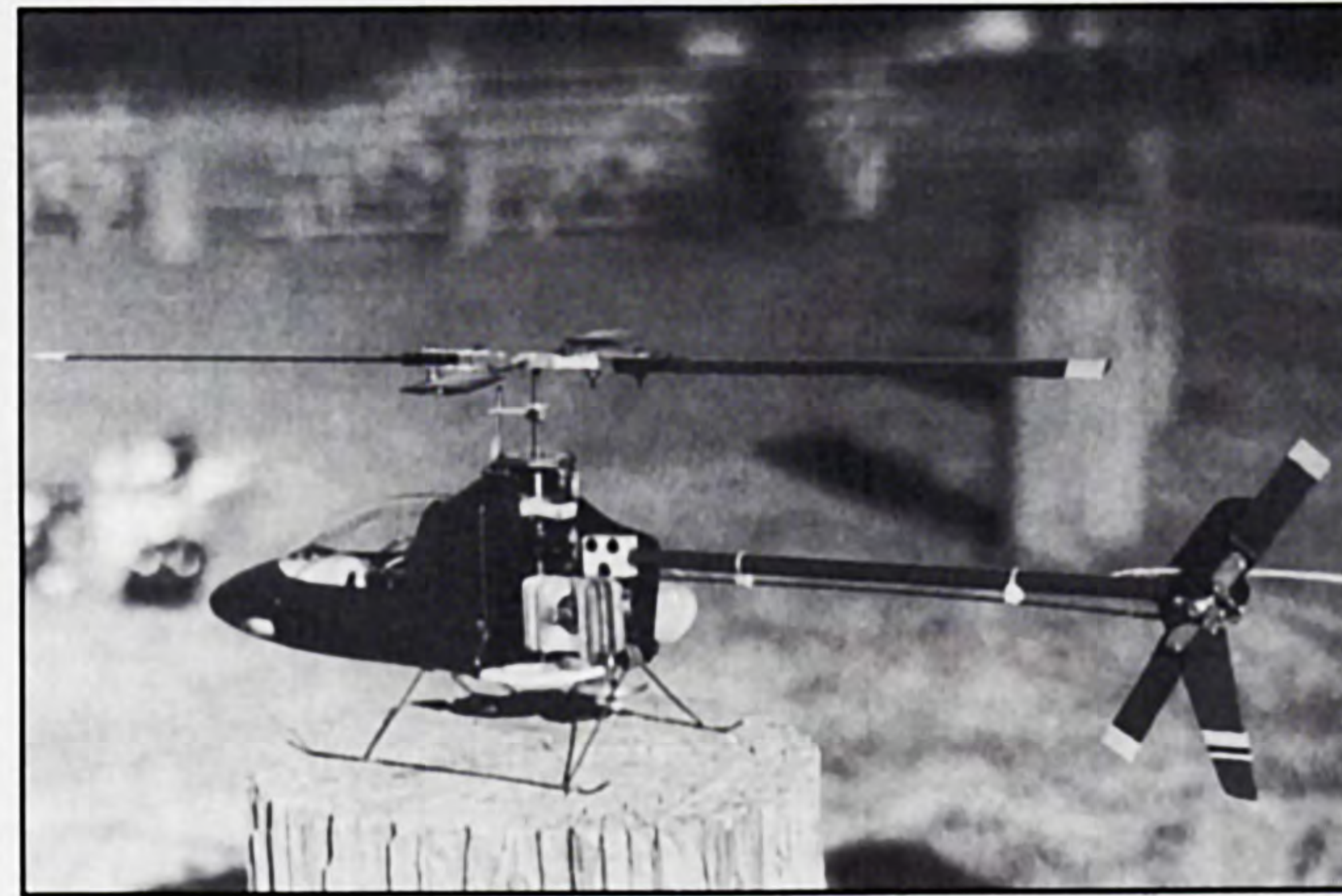
Left: Dave skillfully adjusts the temperature of an overheated Prototype I at our secret test flying site (a parking lot in the Purdue Research Park). Right: Prototype II had an ineffective sheet metal heat sink on the engine and no clutch. The receiver antenna wire hung out the back of a nylon tube running along the tail boom. After shortening the antenna several inches with the tail rotor, we decided to install a whip antenna on Prototype III.
