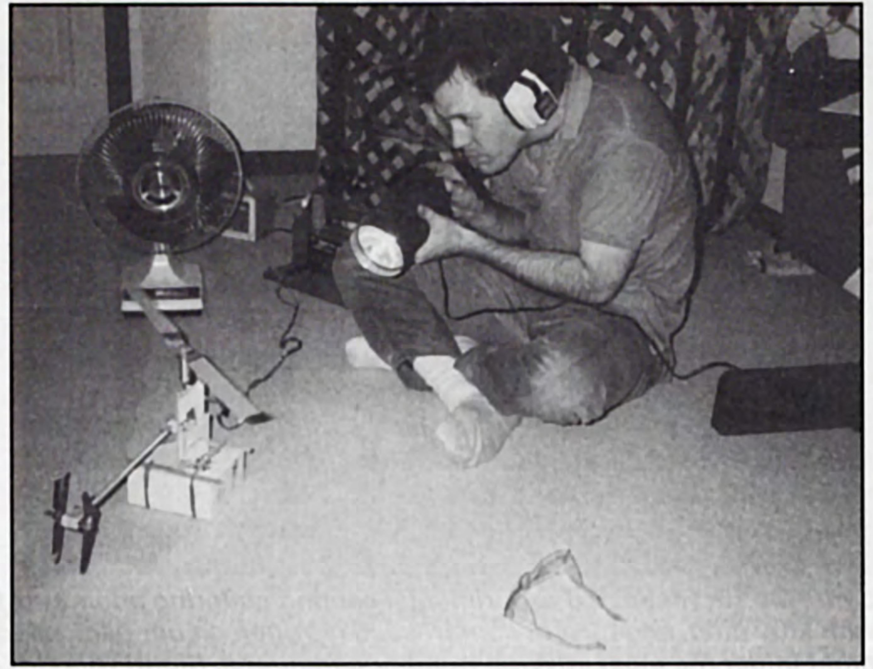
Left: The "rotary glider" concept consisted of large slow moving blades running at 600 to 800 rpm. This apparatus powered by a Dremel motor tool (and held by yours truly) allowed tests to be performed indoors under controlled conditions. Note the two-stage gear reduction to the main rotor, and the torsion spring at the front of the tail tube driving the tail rotor. Right: This test stand (attached with rubber bands to a box weighted with pennies) was powered by an R/C car motor and flight box battery (in background). The fan caused the rotors to blow back, simulating windy conditions. We frequently used a hand-held strobe light to freeze motion when studying rapidly rotating mechanisms.
