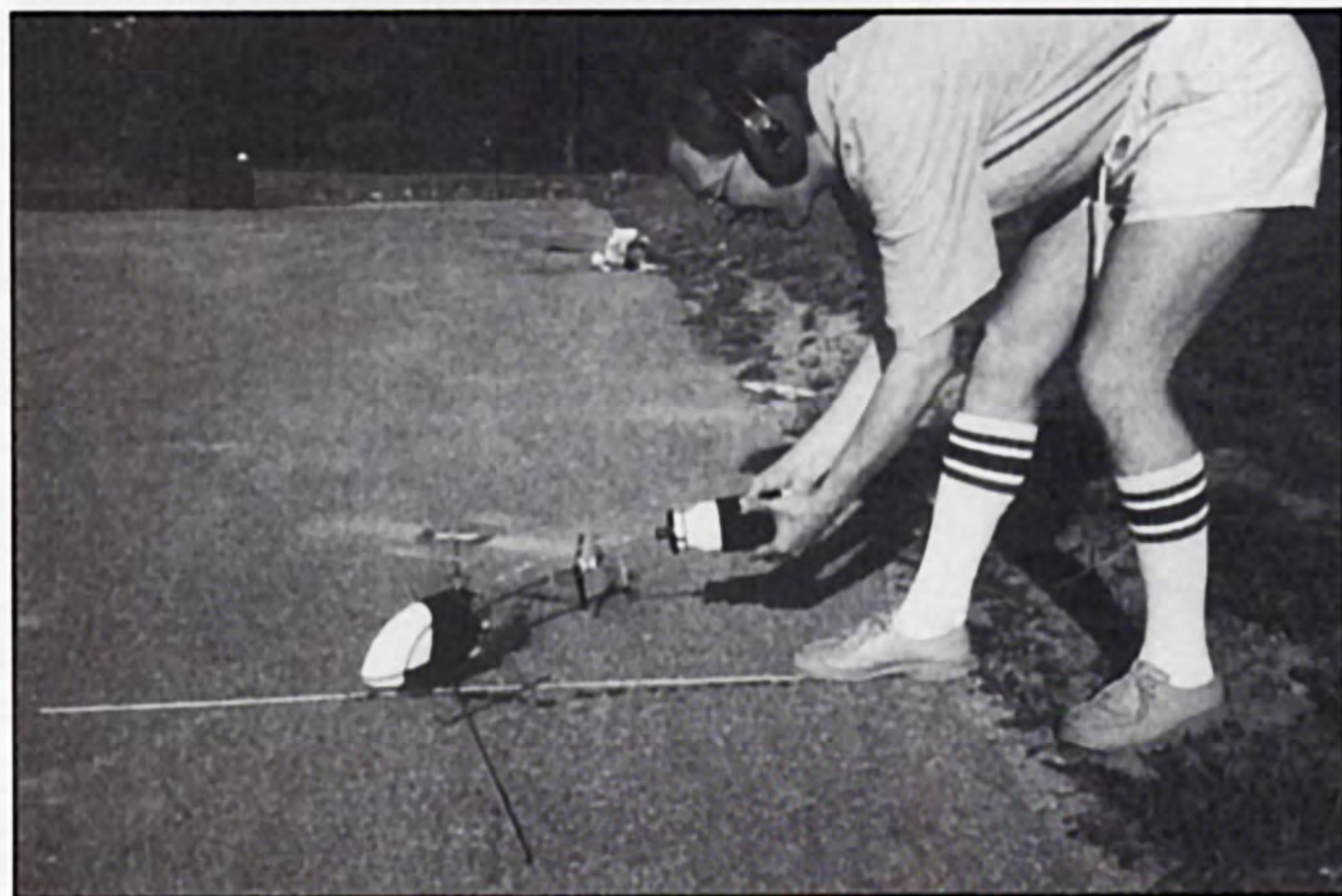
Left: Dave skillfully adjusts the temperature of an overheated Prototype I at our secret test flying site (a parking lot in the Purdue Research Park). Right: Prototype II had an ineffective sheet metal heat sink on the engine and no clutch. The receiver antenna wire hung out the back of a nylon tube running along the tail boom. After shortening the antenna several inches with the tail rotor, we decided to install a whip antenna on Prototype III.
