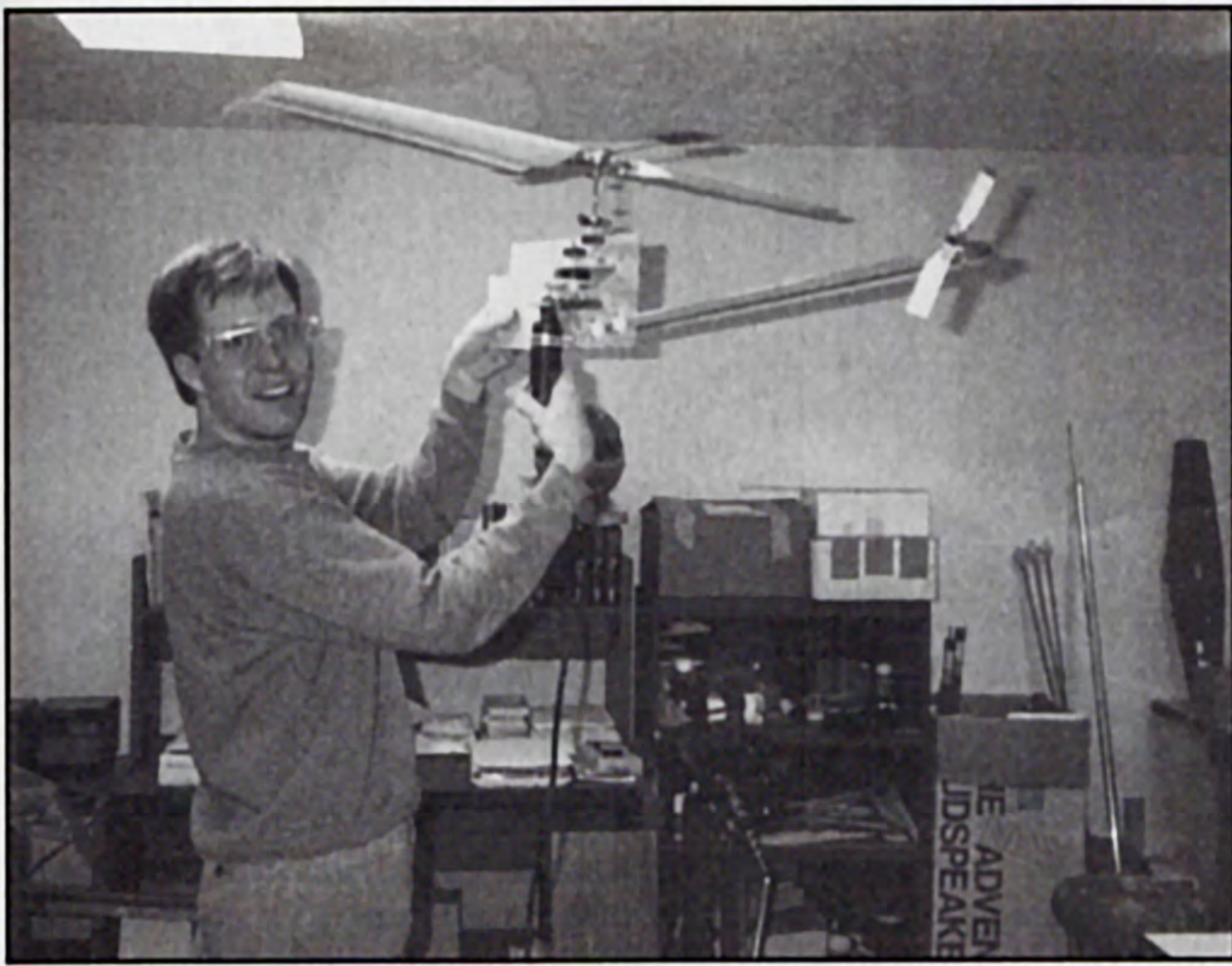
Left: The "rotary glider" concept consisted of large slow moving blades running at 600 to 800 rpm. This apparatus powered by a Dremel motor tool (and held by yours truly) allowed tests to be performed indoors under controlled conditions. Note the two-stage gear reduction to the main rotor, and the torsion spring at the front of the tail tube driving the tail rotor. Right: This test stand (attached with rubber bands to a box weighted with pennies) was powered by an R/C car motor and flight box battery (in background). The fan caused the rotors to blow back, simulating windy conditions. We frequently used a hand-held strobe light to freeze motion when studying rapidly rotating mechanisms.
