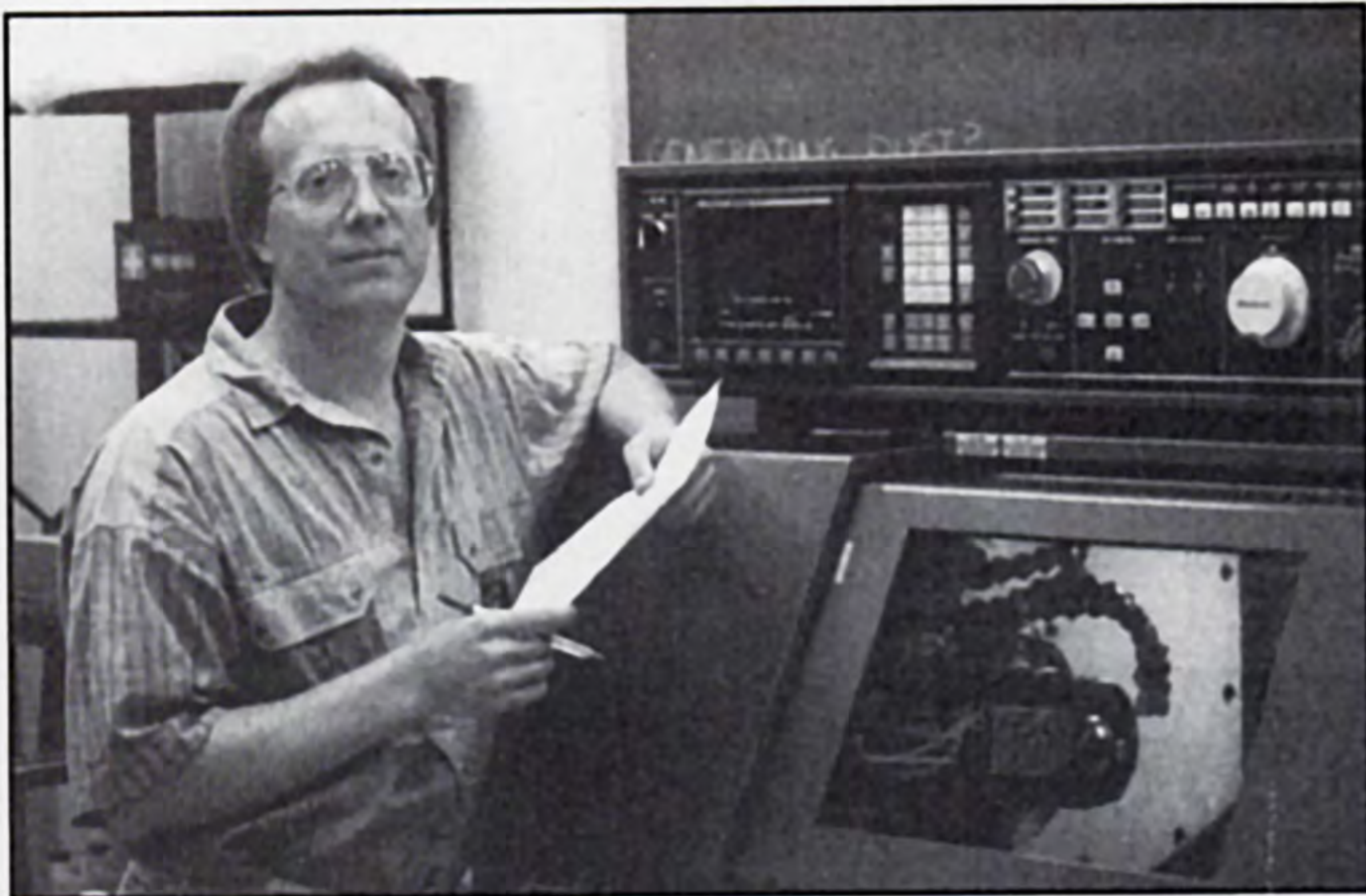
Left: Dave is developing a program for our CNC lathe at the lab. This machine cost more than $100,000.00, and makes heat sinks and other small metal and plastic parts. Right: During an experiment at the Purdue Aerospace Sciences Laboratory, Dave is holding a stick dipped in titanium tetrachloride near the test stand in order to visualize the vortex generated at the tip of the rotor blade. Titanium tetrachloride is a liquid that breaks down into titanium oxide (fine white powder) and hydrochloric acid when exposed to air. Within a few hours of this experiment, all of the exposed steel on the test stand was coated with rust caused by the airborne hydrochloric acid.
