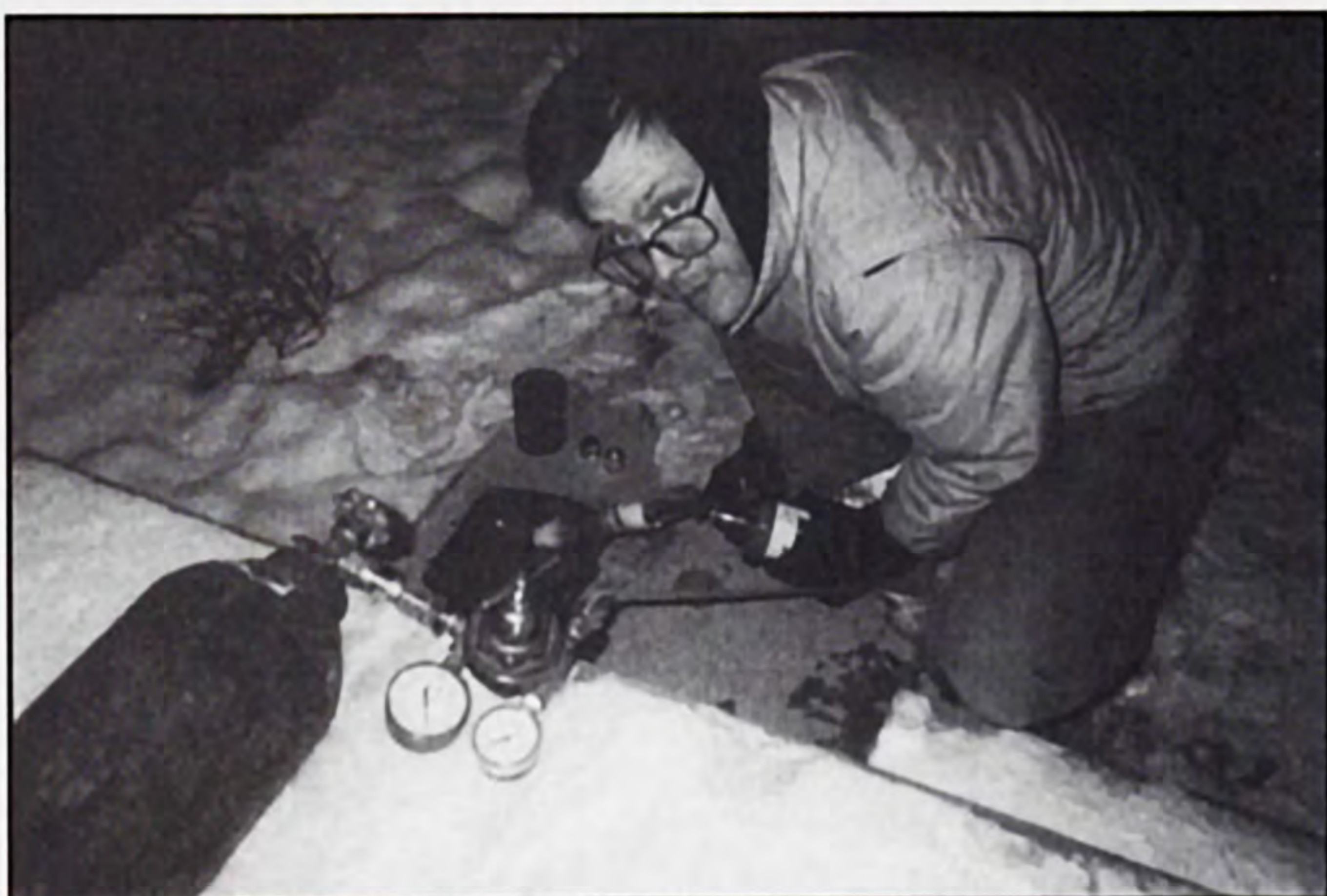
Left: This sophisticated experimental casting/sintering apparatus for making gear molds involved a propane torch, brownie pan lined with kitty litter, and tank of compressed nitrogen on our back patio. We always perform delicate experiments such as this outdoors at night under the most adverse weather conditions. Right: This Cox 049 powered test mechanism preceded Prototype I. The main rotor and tail rotor are fully functional and ready to be mounted to an airframe with radio.
